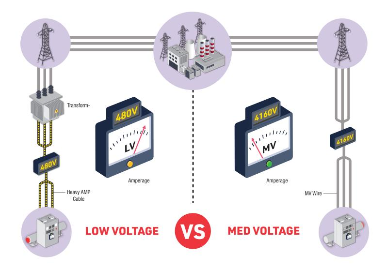
That all recently changed when Chromalox developed and patented the first true medium voltage element rated to a voltage of 7200VAC. Referred to as DirectConnect (see Figure 1), these medium voltage electric heating elements provide a significant advantage over conventional electric designs and bridge the gap from electric technology to fuel fired technology for steam generation and process heating.
