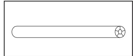
2. **Porcelain Beads** — Listed in table below. Can be used when wiring does not permit straight tubing.
