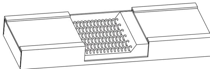
**Refractory is then Compressed to Rock-Hardness** and high density under tremendous hydraulic pressure to maximize heat transfer from coil to sheath. Elements are oven cured at high temperatures to semi-vitrify and mature the refractory.
