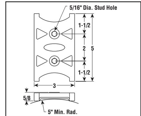
**Clamp 6933** — Use to clamp two strip heaters on 3" centers using 3/8" studs at 5" intervals (PCN 263644).
