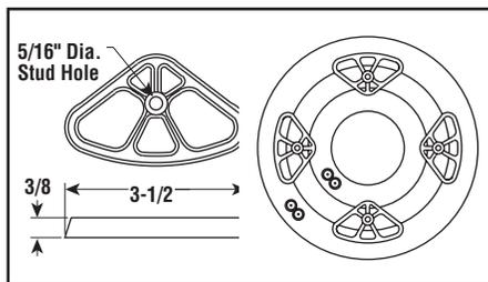
**Clamp 5971** — Use to clamp two strip heaters on 2" centers using 5/16" studs spaced 5" apart (PCN 263636).
