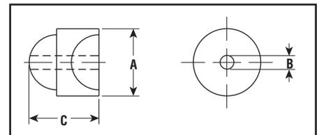
3. When selecting porcelain beads for stranded wire, use next larger gauge wire and use bead for that size (i.e., 10 gauge stranded wire requires a No. 6 bead).
