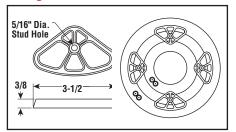
**Clamp 5971** — Use to clamp two strip heaters on 2" centers using 5/16" studs spaced 5" apart (PCN 263636).
