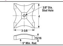
**Clamp 5970** — Use to clamp three strip heaters on 2" centers using 5/16" studs at 5" intervals (PCN 263652).
