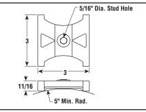
**Clamp 6933** — Use to clamp two strip heaters on 3" centers using 3/8" studs at 5" intervals (PCN 263644).
