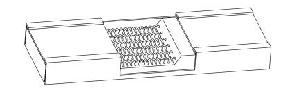
**Refractory is then Compressed to Rock-Hardness** and high density under tremendous hydraulic pressure to maximize heat transfer from coil to sheath. Elements are oven cured at high temperatures to semivitrify and mature the refractory. **Maximum Heat Transfer,** from the instant the element is first energized, is provided by the high emissivity black oxide finish. Elements with shiny surfaces do not transfer heat as well.
