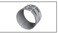
**Fig. 17 –** Splitcase — Allows heater to be opened one time for mounting. Available with any termination or mounting arrangement.
