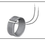
Fig. 3 - Single conductor metal braid over lead wire. Offers most practical solution to abrasion problem. 12" braid with 14" overall length leads are standard.
