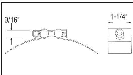
**Fig. 20 Wide Barrel** — 1-1/4" Wide Barrel Assembly Welded to Sheath with 5/16-18 Socket Head Screw
