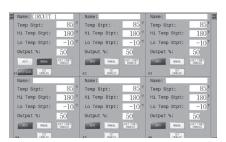
The 10" or 7" Touch Screen Computer provides real time display of process variable, set point, load current, load demand (%), operation mode type, alarm status and alarm type for any 2 or 6 circuits at a time as well as alarm status for all other circuits.
