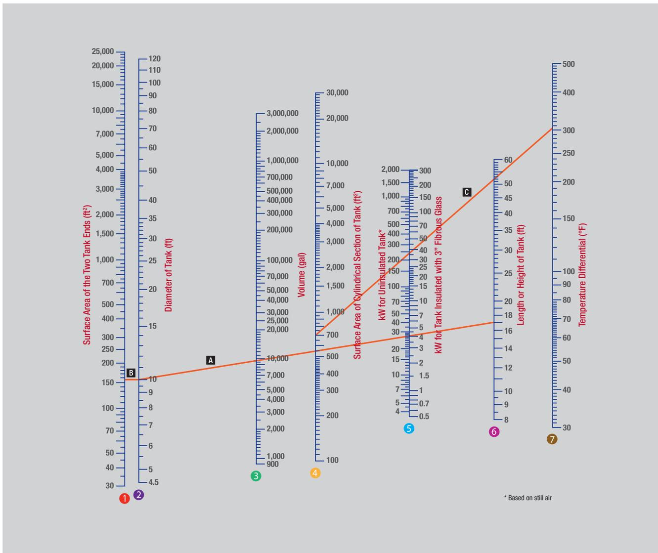
1. Connect 10'-0" on scale ② with 17'-0" on scale ⑥ by a straight line **A**. Intersecting this line with scale ④ will give the surface area of the cylindrical portion of the tank as approximately 550 ft<sup>2</sup>. Note: Intersection of line **A** with scale ③ will show tank volume in gallons. (This is often helpful because the dimensions of the tank can be approximated if only the volume is known.)
