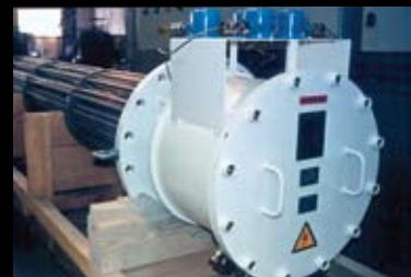
Crude oil heater.
