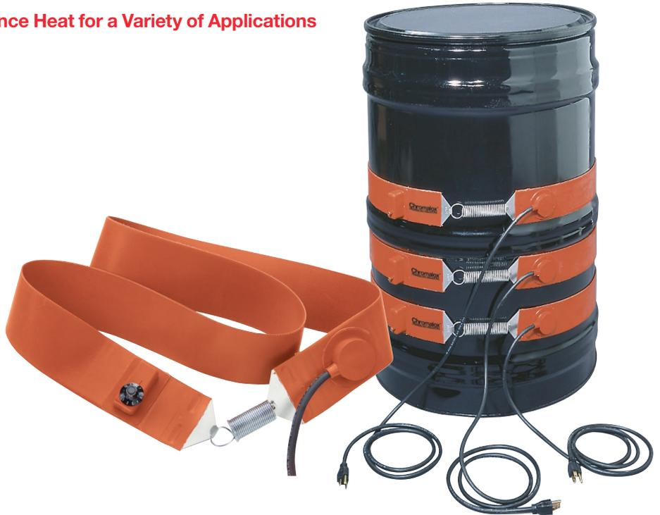
Chromalox SLDH silicone-rubber-insulated drum heaters are designed to provide low-watt-density electrical resistance heat to the contents of drums for freeze protection, melting of low-melting-point solids, viscosity control of fluids, and temperature maintenance of materials while in use.
