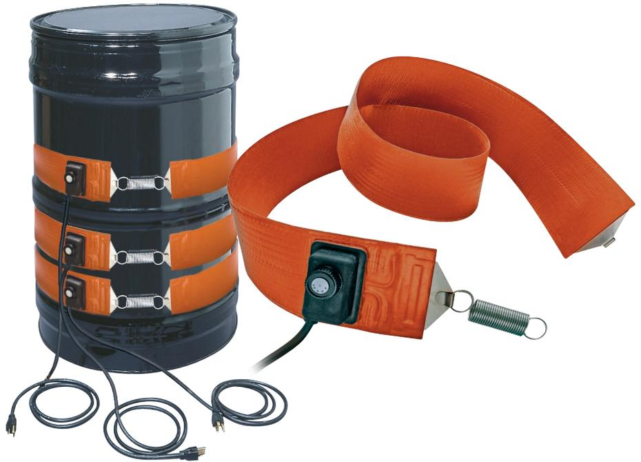
Chromalox PHD heavy-duty fiberglass woven drum heaters are constructed of fiberglass-insulated resistance wire woven into a mesh blanket and then encased in layers of silicone rubber. Like Chromalox SLDH silicone-rubber-insulated drum heaters, PHD fiberglass
