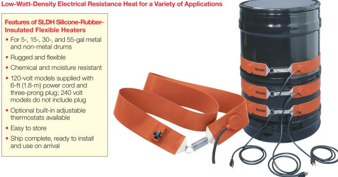
Chromalox SLDH silicone-rubberinsulated drum heaters are designed to provide low-watt-density electrical resistance heat to the contents of drums for freeze protection, melting of lowmelting-point solids, viscosity control of fluids, and temperature maintenance of materials while in use.
