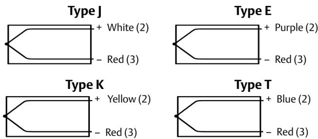
**Figure 2-5. Rosemount 185 Thermocouple Lead Wire Configurations**
