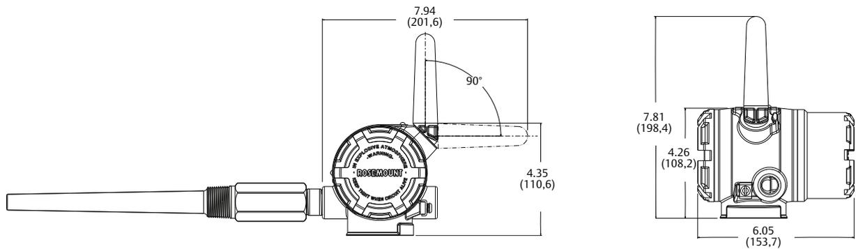
Direct mounted temperature sensor specified separately (see ordering option code XA).
