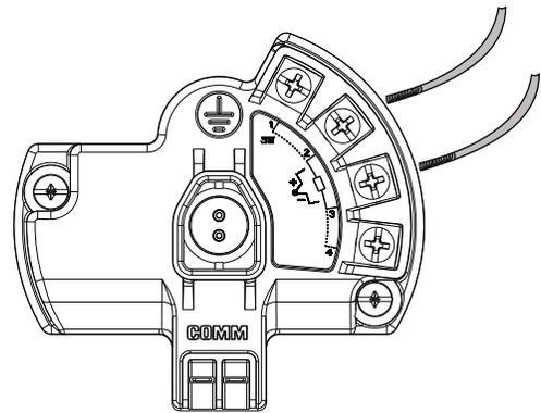
248 Wireless Sensor Connections Diagram
