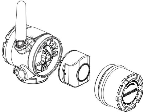
6. Close the housing cover and tighten to safety specification. Always ensure a proper seal by installing the electronics housing covers so that metal touches metal, but do not over tighten.
