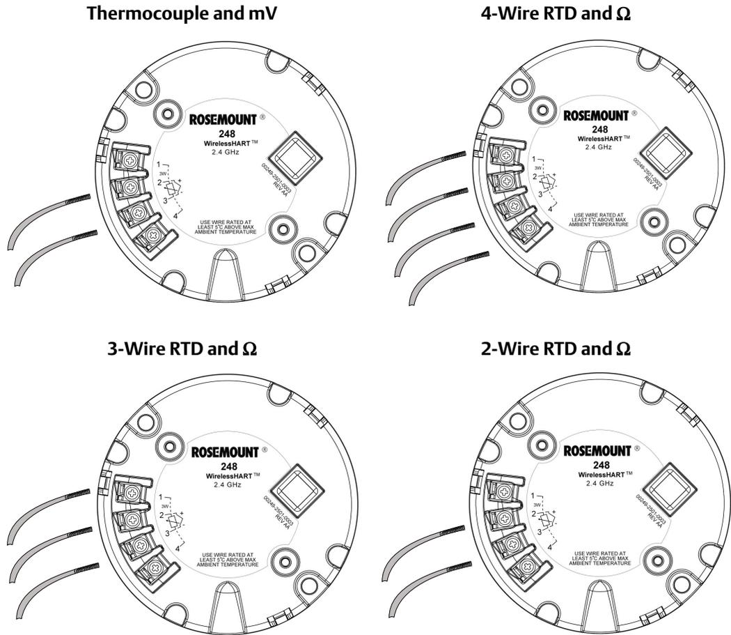
248 Wireless Sensor Connections Diagram
