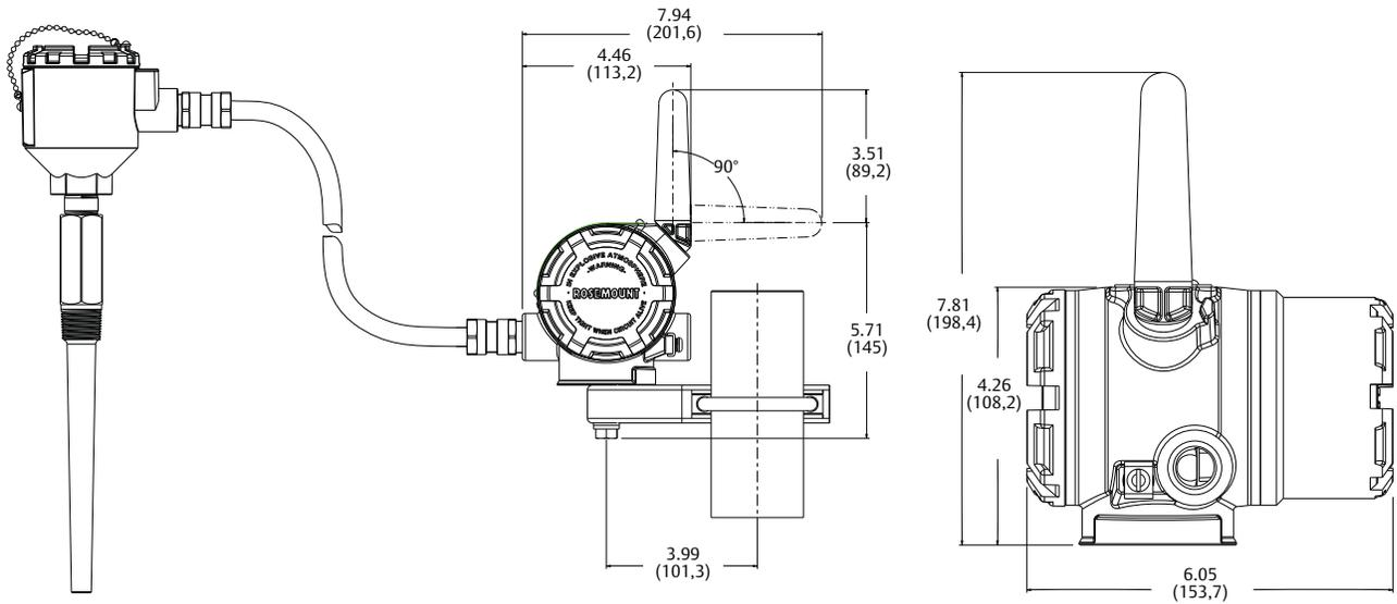
Remote mounted temperature sensor specified separately.
