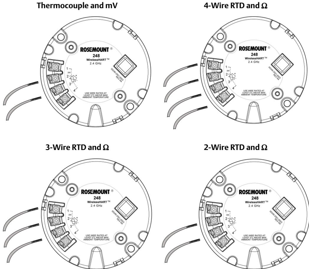
248 Wireless Sensor Connections Diagram
