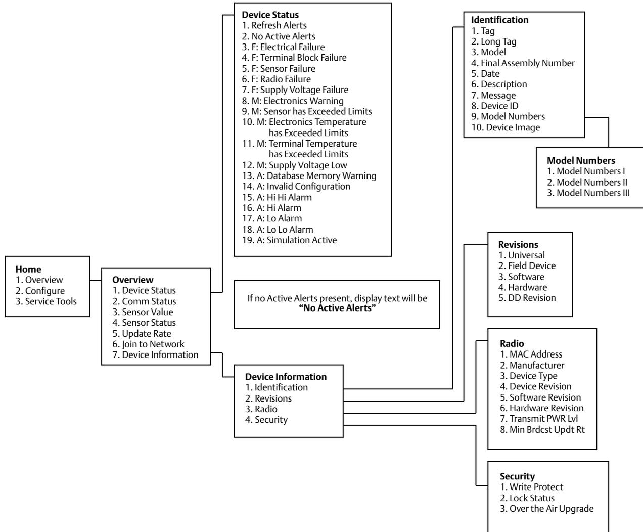
Figure 2-11. Field Communicator Menu Tree: Configure (Polymer Housing)
