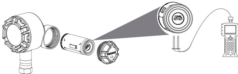
Figure 2-9. Field Communicator Connections (Aluminum Housing)
