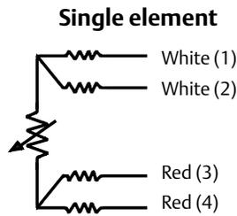
**Figure 2-4. Rosemount 183 Thermocouple Lead Wire Configuration**
