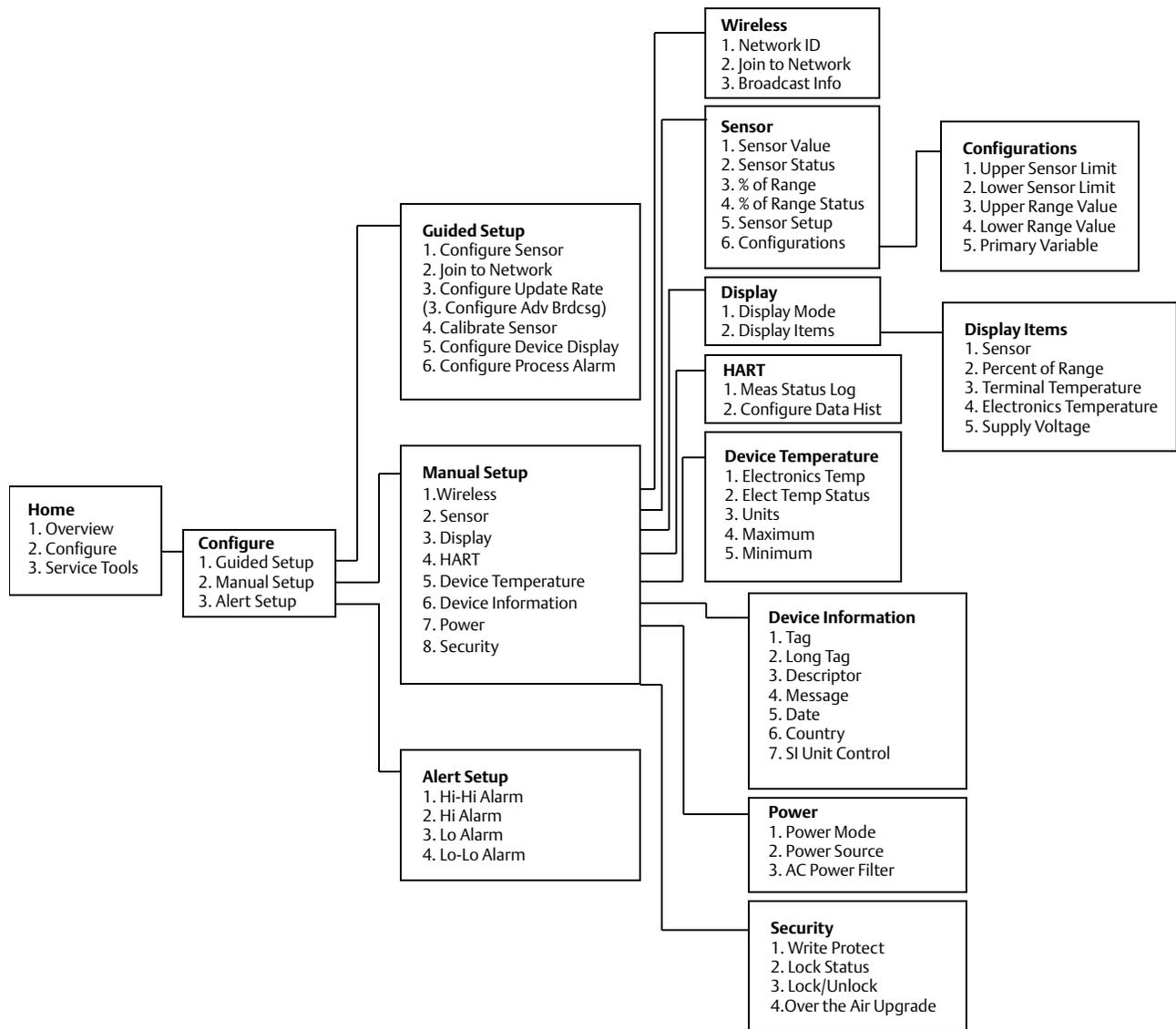
Figure 2-12. Field Communicator Menu Tree: Service Tools (Polymer Housing)
