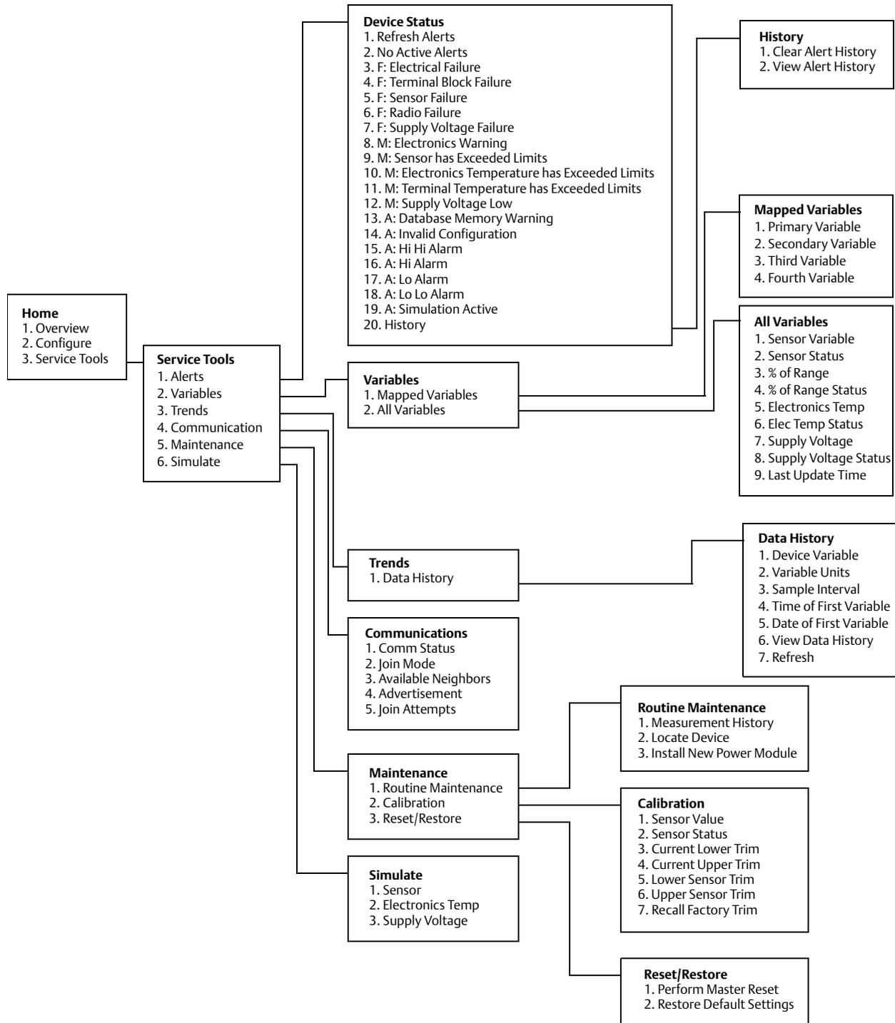
Figure 2-13. Field Communicator Menu Tree (Aluminum Housing)
