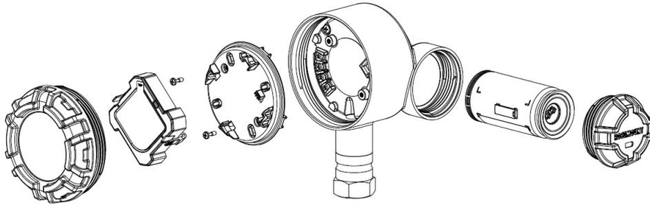
4. Attach the sensor to the 248 Wireless housing using the threaded conduit entry. Be sure to use an approved thread sealant on all connections.
