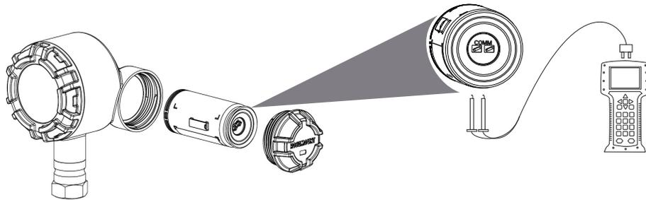
**Figure 2-7. Field Communicator Connections (Aluminum Housing)**
