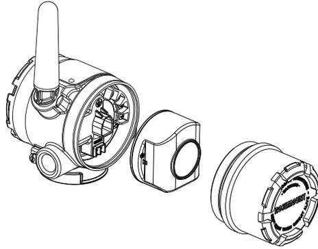
5. Close the housing cover and tighten to safety specification. Always ensure a proper seal by installing the electronics housing covers so that metal touches metal, but do not over tighten.
