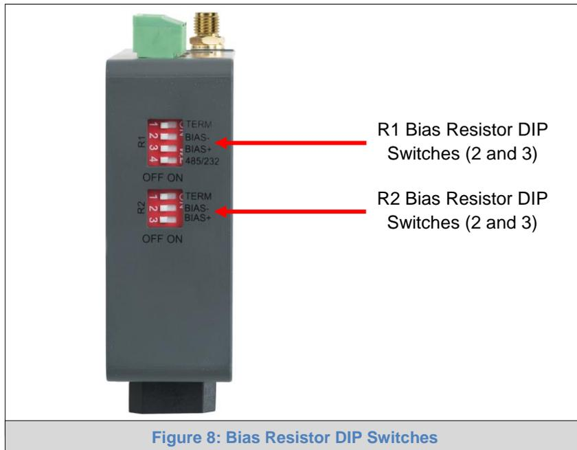
Figure 8: Bias Resistor DIP Switches
