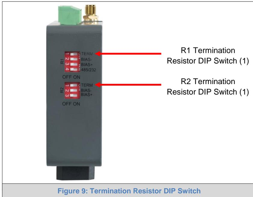
Figure 9: Termination Resistor DIP Switch
