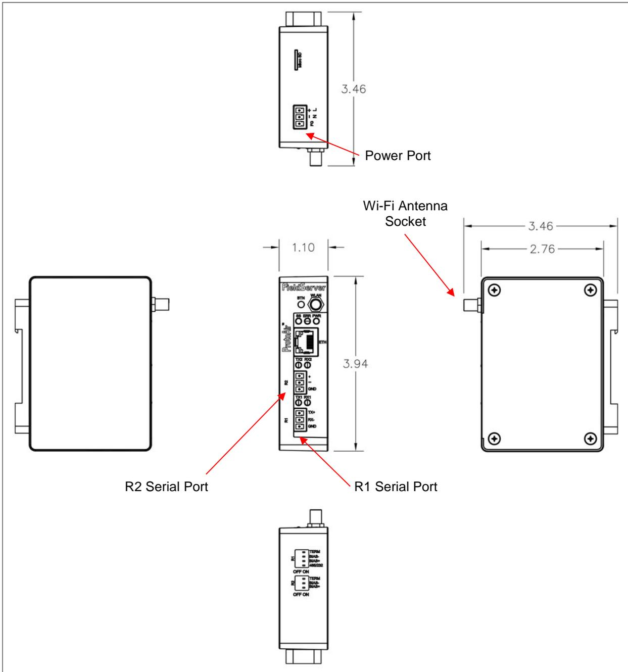
Figure 53: ProtoAir FPA-W44 Dimensions
