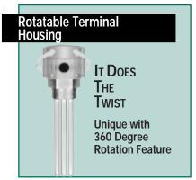
The NEMA 1 terminal enclosure of the Chromalox screw plug heater is fully rotatable. This patented feature allows 360° rotation of the terminal enclosure (270° rotation for heaters with thermostat). Thus, you are able to rotate the enclosure (housing) to face the electrical conduit connection after the heater has been properly installed.
