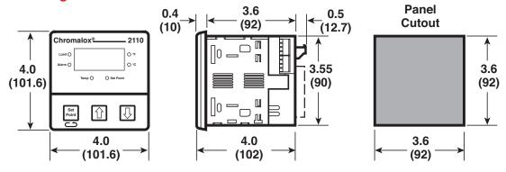
All dimensions in inches (mm) \* With alarm option or S2 output
