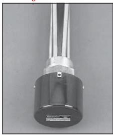
Screw Plug Immersion Heaters consist of hairpin bent tubular elements brazed or welded into a screw plug and provided with terminal enclosures for electrical connections. Screw plug immersion heaters are screwed directly through a threaded opening in a tank wall or into a matching half coupling.
