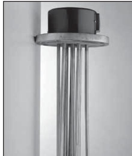
Flanged Immersion Heaters consist of hairpin bent tubular elements welded or brazed into a flange and provided with terminal enclosures for electrical connections. Flange heaters are installed by bolting to a matching flange welded to the tank wall or nozzle.
