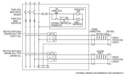
Ambient Sensing Three Phase 208/120 4-Wire or 480/277 4-Wire
