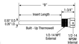
Note: When fitting thermocouple to thermowell, probe length is the same as "B" dimension on thermowell.
