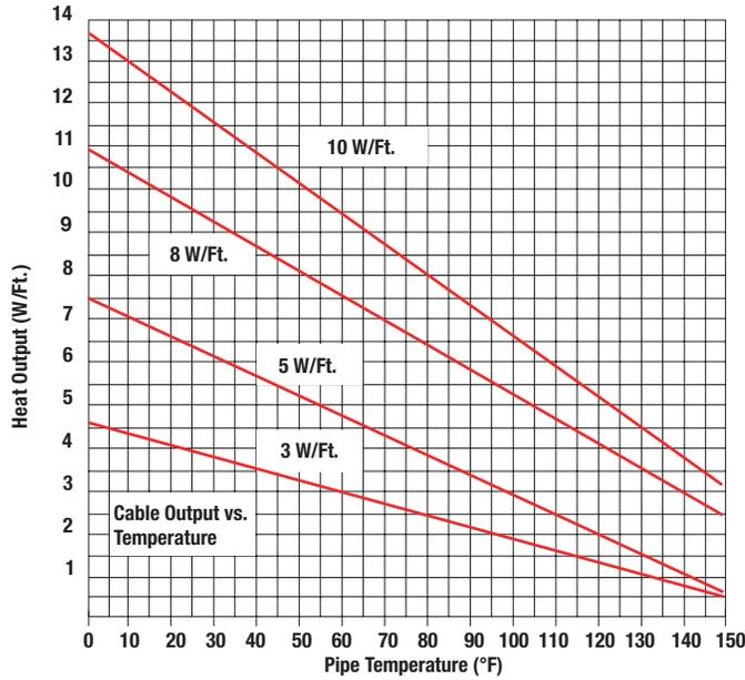
**Note 1** — Thermal output is determined per IEEE 515-2011 Standard for testing, design installation, and maintenance of electrical resistance heat tracing section 4.1.11 Method C.
