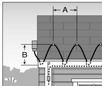
2. Add the total gutter length and the total downspout length to the figure calculated in step 1 to get the total length of cable required.
