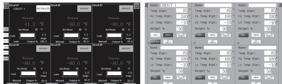
The 7" or 10" Touch Screen Computer provides real time display of process variable, set point, load current, load demand (%), operation mode type, alarm status and alarm type for any 2 or 6 circuits at time as well as alarm status for all other circuits.
