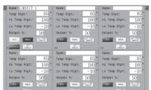
The 10" or 7" Touch Screen Computer provides real time display of process variable, set point, load current, load demand (%), operation mode type, alarm status and alarm type for any 2 or 6 circuits at time as well as alarm status for all other circuits.
