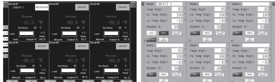
The 10" or 7" Touch Screen Computer provides real time display of process variable, set point, load current, load demand (%), operation mode type, alarm status and alarm type for any 2 or 6 circuits at time as well as alarm status for all other circuits.
