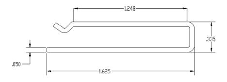
Note: CHTB comes with the above bracket. Adhesives, junction boxes, conduits and heating cable are provided by separately. Appropriate control and monitoring systems should be used with the CHTB system. For heat trace specs see appropriate heat trace datasheet.
