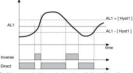
For AL1 = symmetrical inverse absolute alarm with Hyst1, AL1 t = 5 For AL1 = symmetrical direct absolute alarm with Hyst1, AL1 t = 4 Minimum hysteresis = 2 scale points
