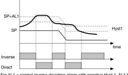
For AL1 = normal inverse deviation alarm with negative Hyst 1, AL1 t = 3 For AL1 = normal direct deviation alarm with negative Hyst 1, AL1 t = 2
