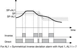
For AL1 = Symmetrical inverse deviation alarm with Hyst 1, AL1 t = 7 For AL1 = Symmetrical direct deviation alarm with Hyst 1, AL1 t = 6
