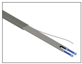
Slide one end of each of the two insulated barrel connectors over the bare portion of the conductors. Crimp the barrel connectors on using a crimping tool.
