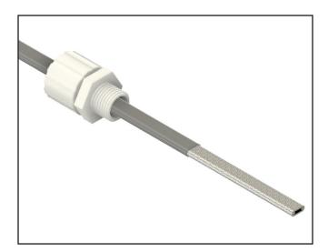
**3.** Score the cable outer jacket 3 ½" from the cable end, being careful not to damage the braid or the base cable insulation. Remove the jacket to expose the braid.
