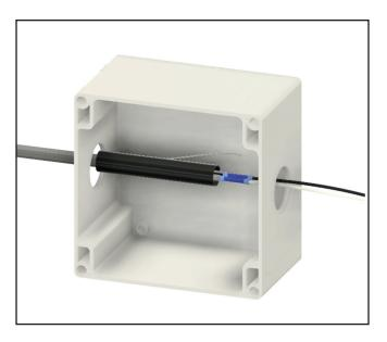
**10.** Insert the bared portion of the power leads into the other end of the insulated barrel connectors and crimp them.
