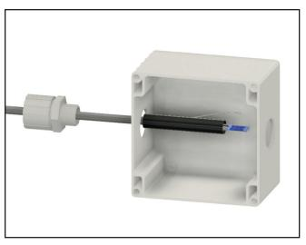
**8.** Insert the entire assembly into a NEMA 4 or 4X Electrical Junction Box (purchased separately).
