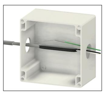
**12.** Insert the end of the braided pigtail into one end of the uninsulated (silver) barrel connector and crimp it. Insert the stripped end of the ground wire into the other end of the barrel connector and crimp it.
