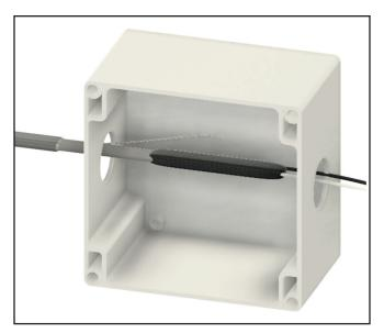
11. Center the 3" long heat shrink tube over the connection. Apply heat evenly to shrink tubing around the heating cable, barrel connectors and power leads. While the shrink tubing is still hot, gently squeeze the shrink tubing between the power leads with needle-nose pliers and hold until cool. The shrink tubing must remain visibly sealed when the pliers are removed. If the tubing does not remain sealed, reheat the tubing and try again
