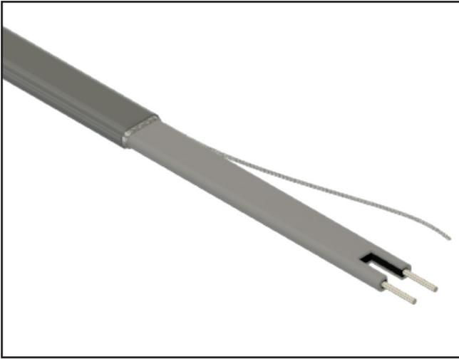
5. Using standard electrical cutters, cut a 3/4" long notch out of the cable, between the two conductor wires. Bare a 3/8" length of each conductor by stripping off the outside insulation and the inner black core material.
