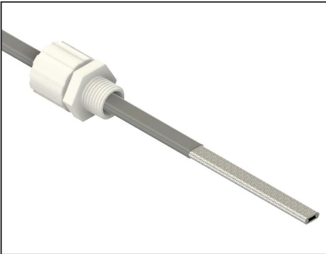
3. Score the cable outer jacket 3 1/2" from the cable end, being careful not to damage the braid or the base cable insulation. Remove the jacket to expose the braid.
