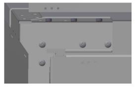
The ground bar link that connects the ground bars in the IEC sections either side of the shipping spilt will be mounted such that it faces into the section.
