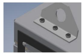
IEC sections must be brought together, and the fasteners (and any associated washers) must be installed from the inside of the section to the left of the slit through into holes where the fasteners were originally installed.
