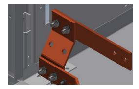
It should be detached from the vertical copper stub that it is attached to, turned through 180 degrees, and reassembled such that it passed through the slot in the adjacent steelwork.
