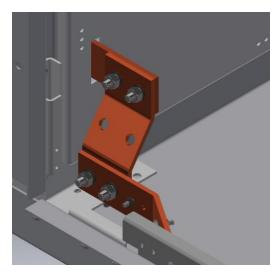
It should be reconnected to the vertical stub it was removed from, and to the equivalent vertical stub in the section to the left of the shipping split with the hardware provided. Tighten the nuts 19.4lbs ft [26.3 Nm].
