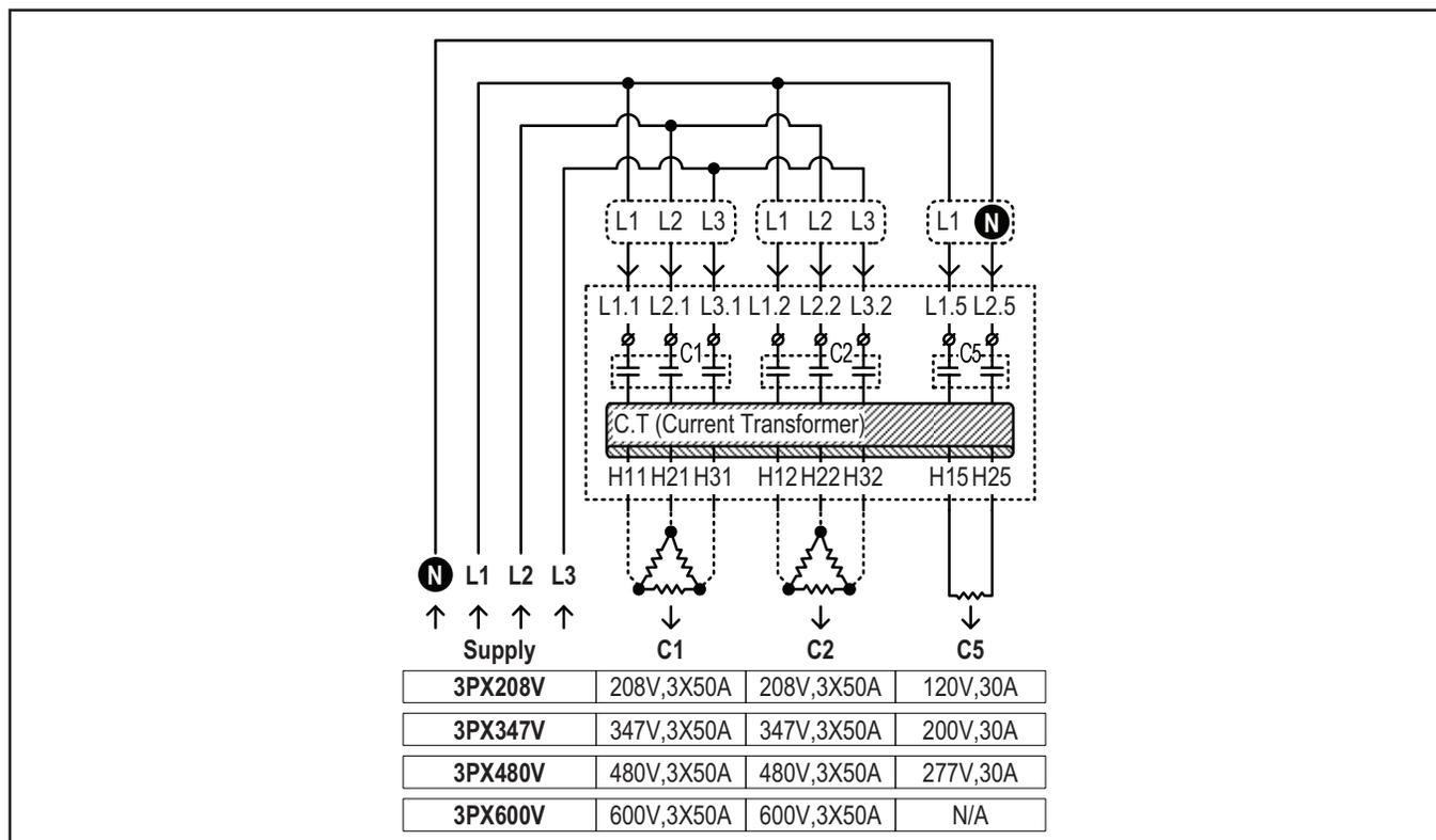
**Note:** Contactors 1 and 2 can be connected to any combination of 1 or 3 (triangle transform) heaters with and without Neutral.
