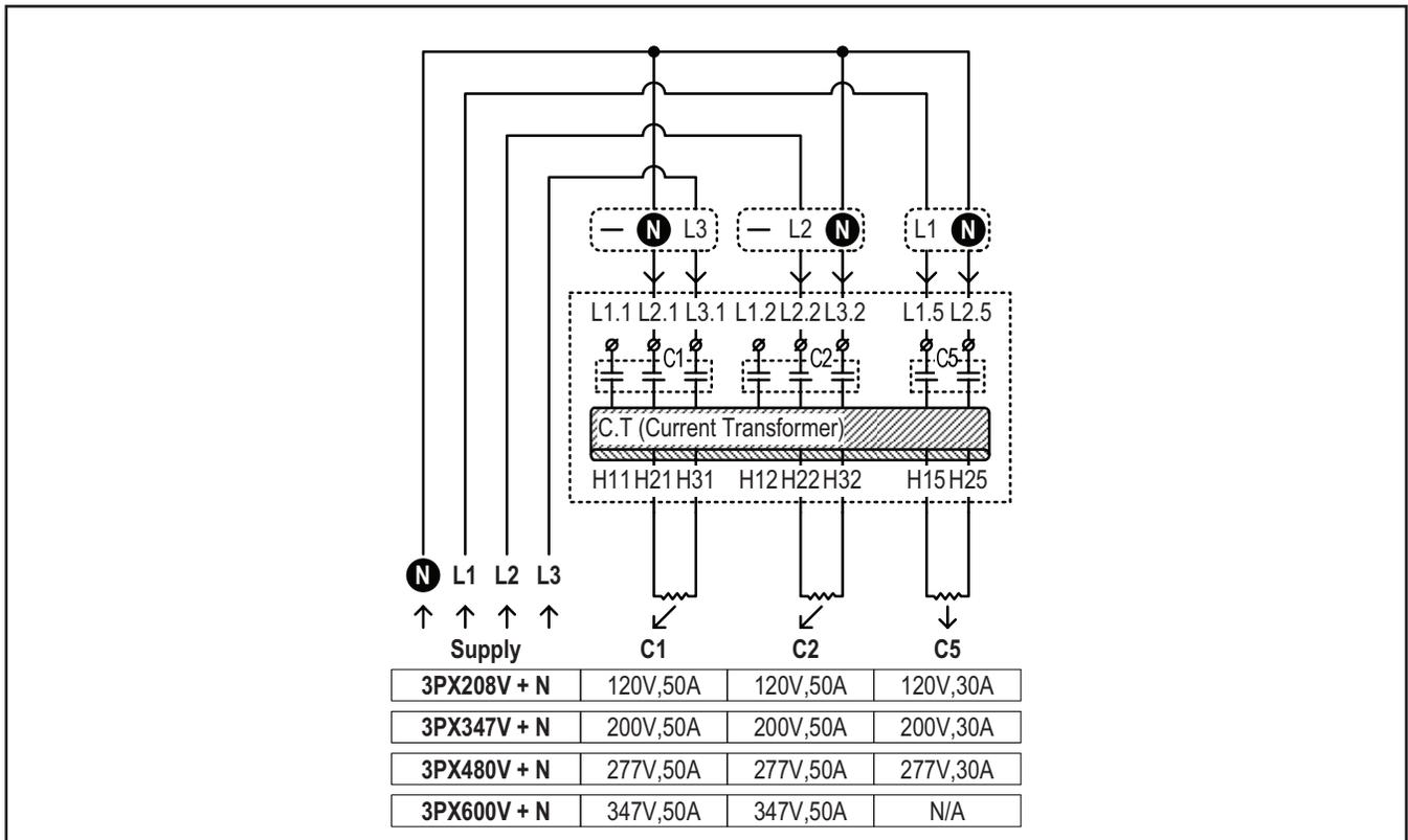
**Note:** Contactors 1 and 2 can be connected to any combination of 1 or 3 (triangle transform) heaters with and without Neutral.
