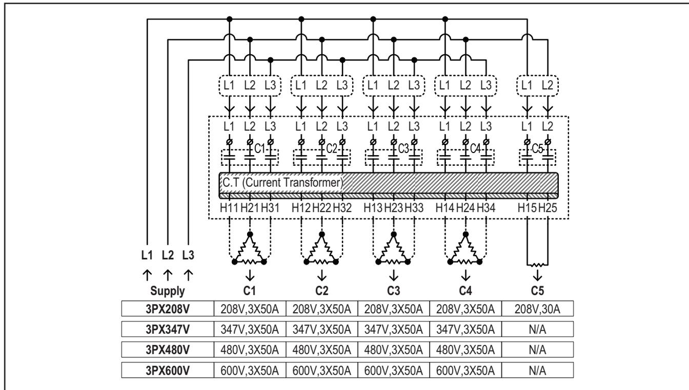
**Note:** Contactors 1 and 2 can be connected to any combination of 1 or 3 (triangle transform) heaters.
