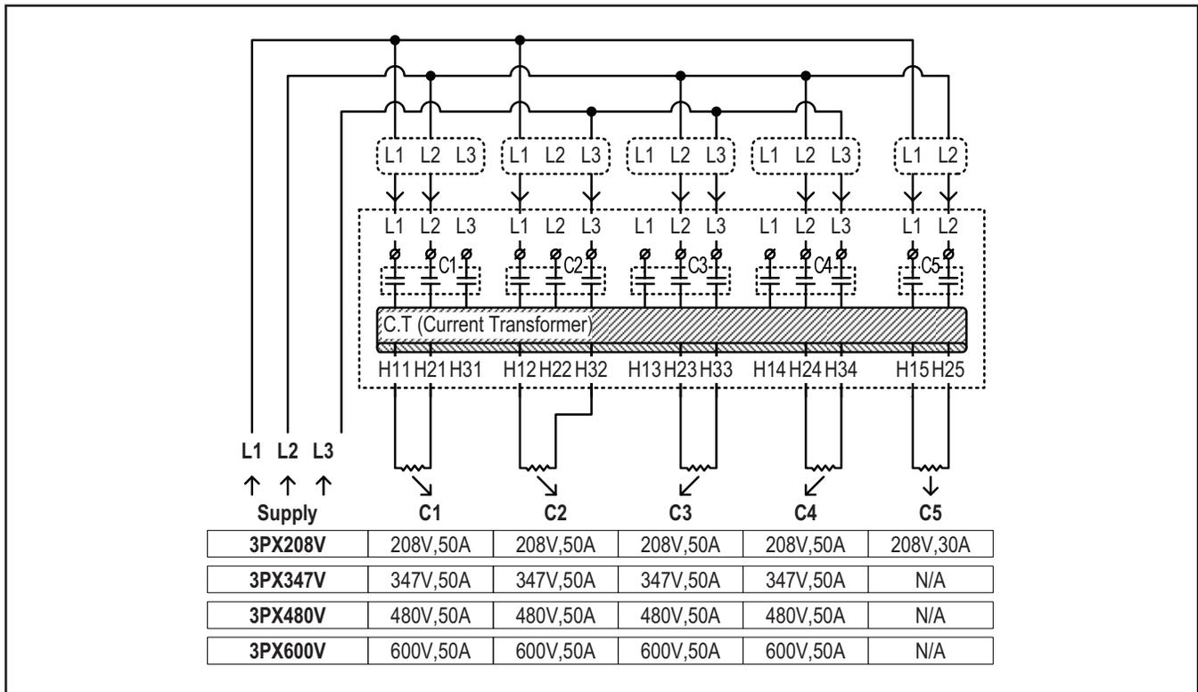
**Option 2:** 3 heaters per contactors C1, C2, C3 & C4 (triangle transform) & 1 heater per contactor C5
