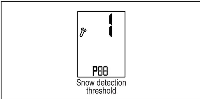
1. Press the [SELECT] and [+] buttons simultaneously.
