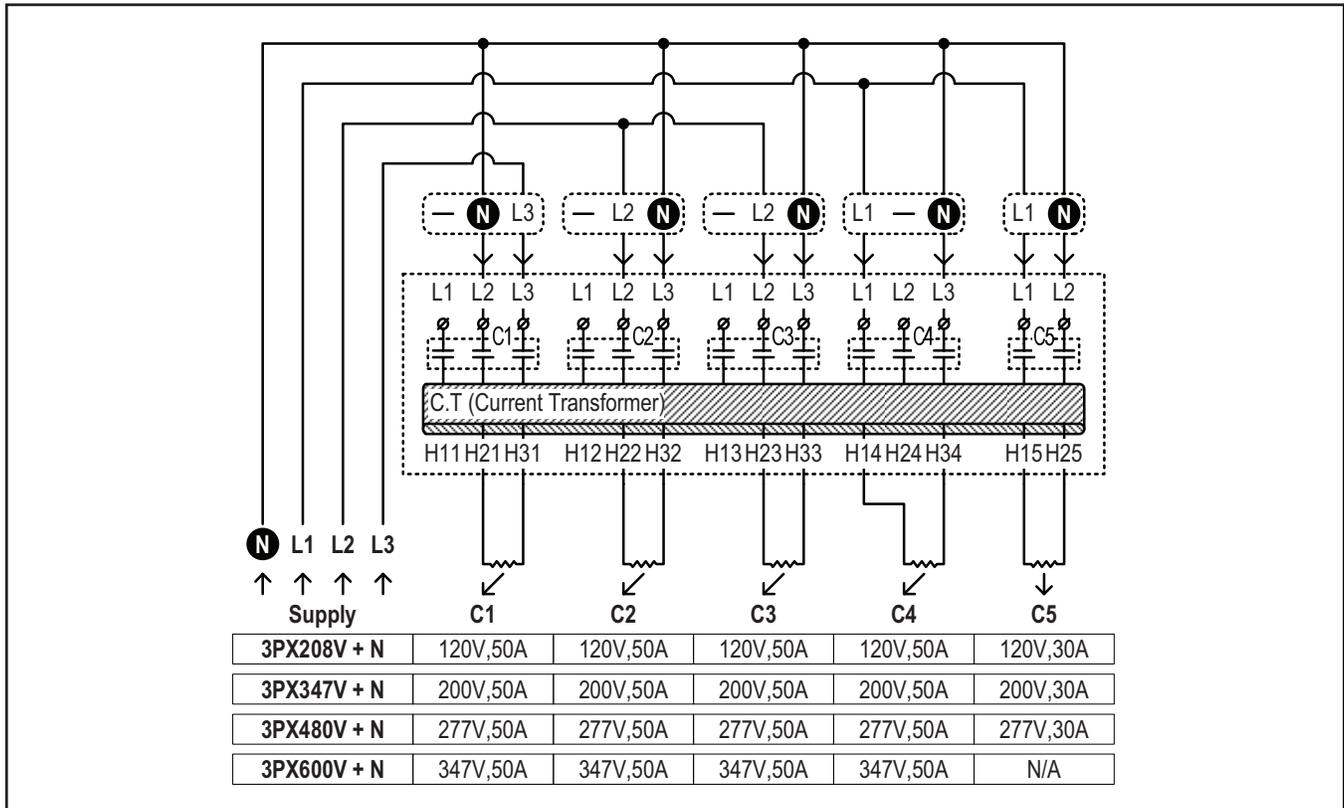
**Note:** Contactors 1,2,3 and 4 can be connected to any combination of 1 or 3 (triangle transform) heaters with and without Neutral.
