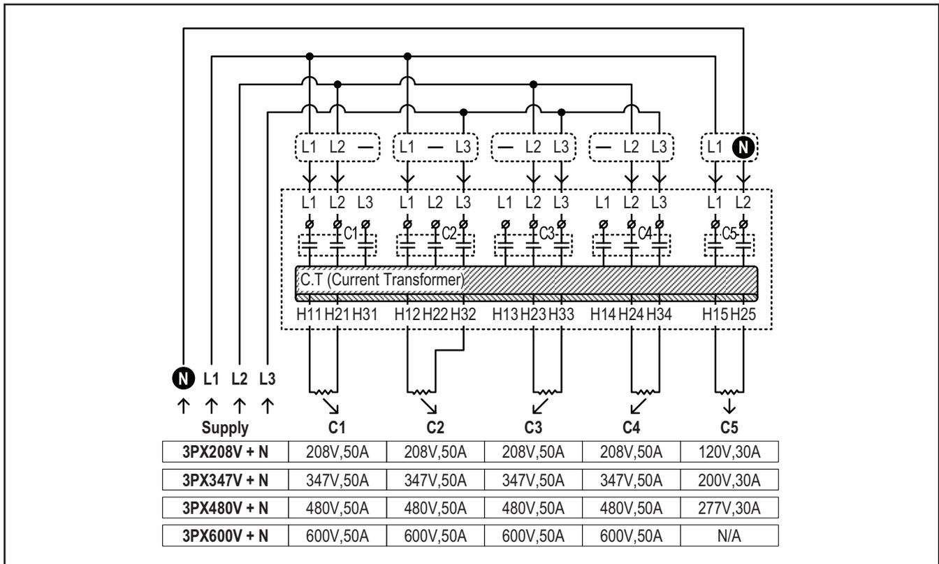
**Option 2:** 3 heaters per contactors C1, C2, C3 & C4 (triangle transform) & 1 heater per contactor C5
