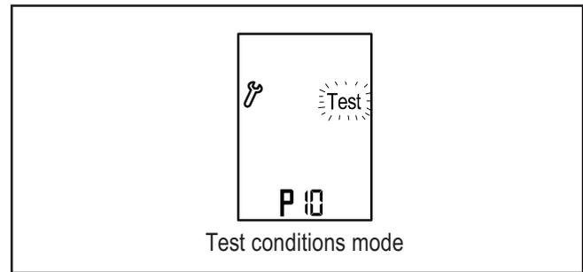
Turn ON test conditions to check the functionality of the system regardless of sensors parameters (i.e. during the summer).
