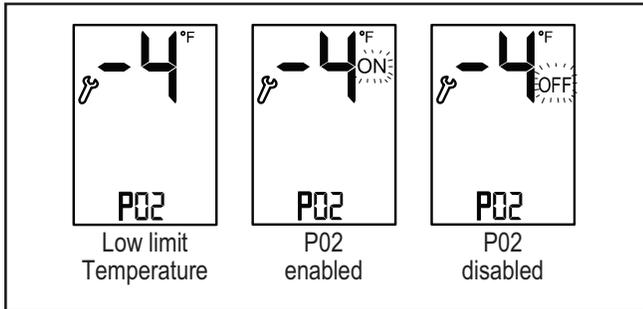
1. Press the [SELECT] and [+] buttons simultaneously.
