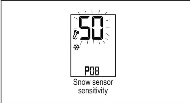
1. Press the [SELECT] and [+] buttons simultaneously
