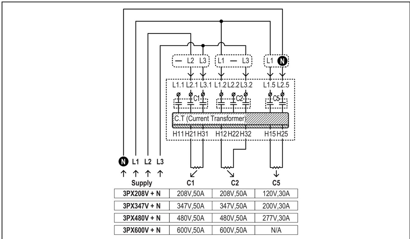
**Option 2: 3 heaters per contactors C1 & C2 (triangle transform) & 1 heater per contactor C5**
