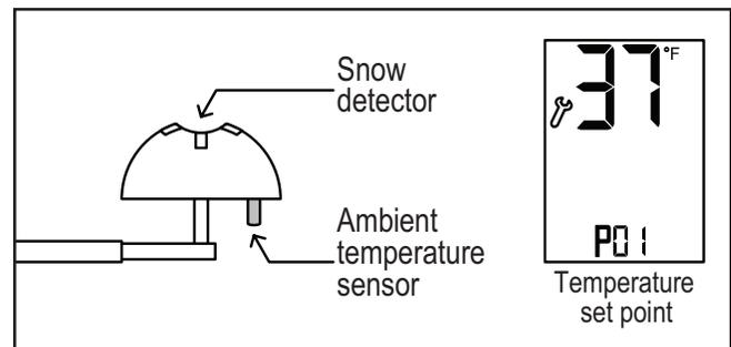
As long as the ambient temperature is lower than the temperature set point P01, the Controller will turn ON upon receiving a positive snow signal from the snow detector.
