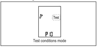
Turn ON test conditions to check the functionality of the system regardless of sensors parameters (i.e. during the summer).
