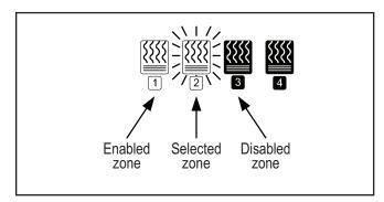
With all heaters enabled: Each heater will be ON for 15 minutes (60/4=15).
