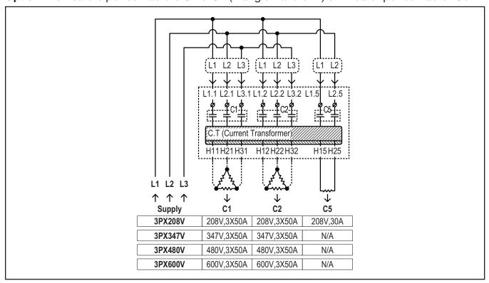
**Note**: Contactors 1 and 2 can be connected to any combination of 1 or 3 (triangle transform) heaters. **Example:** Contactor C1 can be connected to 3 heaters (triangle transform) and contactor C2 can be connected to 1 heater.
