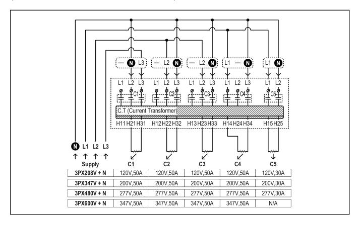
Note: Contactors 1,2,3 and 4 can be connected to any combination of 1 or 3 (triangle transform) heaters with and without Neutral.
