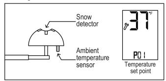
As long as the ambient temperature is lower than the temperature set point P01, the Controller will turn ON upon receiving a positive snow signal from the snow detector.
