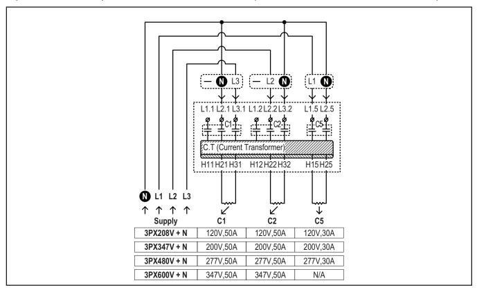
**Note:** Contactors 1 and 2 can be connected to any combination of 1 or 3 (triangle transform) heaters with and without Neutral. **Example:** Contactor C1 connected to 3 heaters (triangle transform) and contactor C2 connected to 1 heater.
