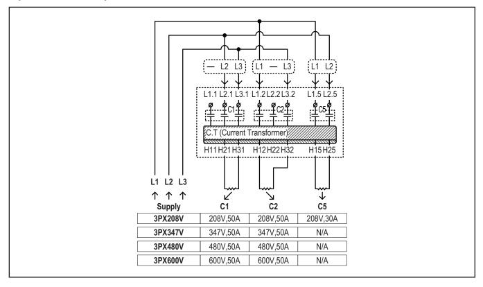
Option 2: 3 heaters per contactors C1 & C2 (triangle transform) & 1 heater per contactor C5
