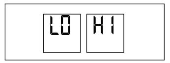
The system will continue to operate using constant predefined values. In addition, the display will alternate between "LO" and -11°F/-24°C for low temperature readings, and between "HI" and 55°F/13°C for high temperature readings.
