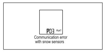
The system will use readings from snow sensor 1 instead of the missing readings from the faulty snow sensor.
