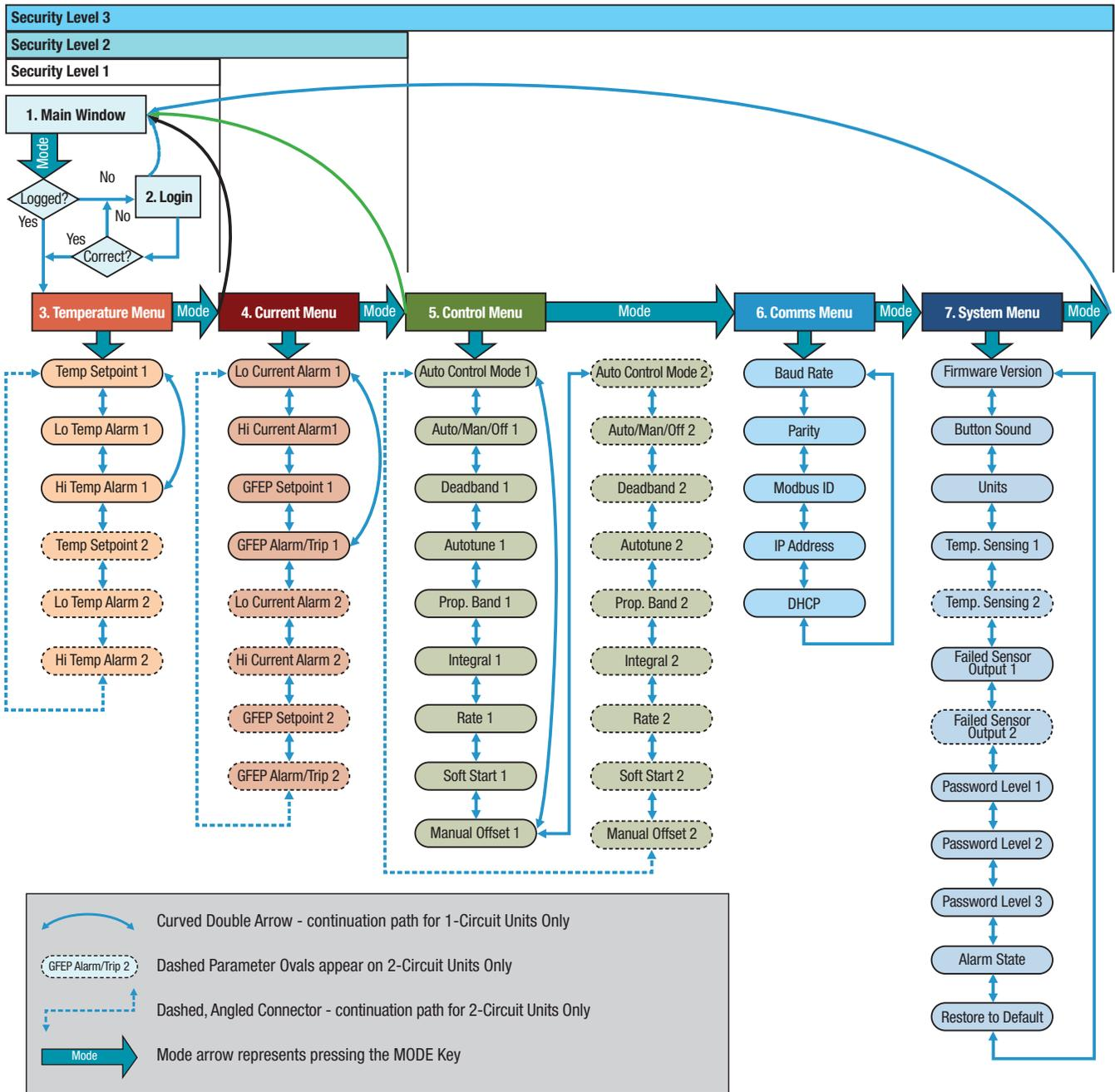
The horizontal security level bars, which are above the CTC Menu & Parameter navigation map, illustrate the available menus within that security level. The Main Window is presented when the **MODE** button is selected
