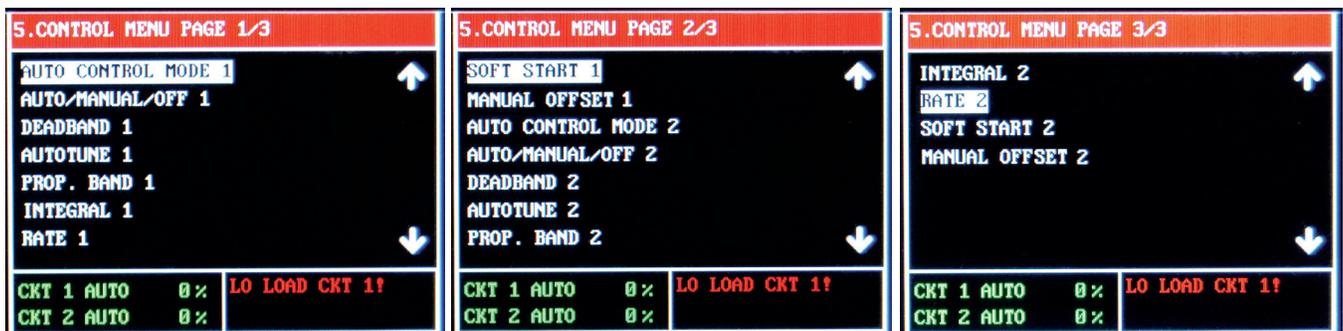
The Control Menu provides access to the types of Automatic Control, Mode of Operation, the parameters which influence the control algorithms and the Soft Start function: Auto Control Mode, Auto/Manual/Off Control, Deadband, Autotune, Proportional Band, Integral, Rate (Derivative), Soft Start function and Manual Offset.
