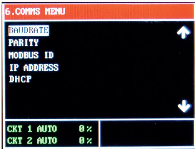
The Comms Menu provides access to the settings for Serial Communications, Modbus RTU/RS-485 or the optional TCP/Ethernet Communications. These communications settings include: Baud Rate, Parity, Modbus ID, IP Address and DHCP.
