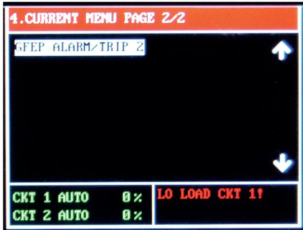
The Current Menu provides access to the current and GFEP based parameters: Low Current Alarm, High Current Alarm, GFEP Setpoint & GFEP Alarm/Trip for Circuits 1 and 2 (when available).
