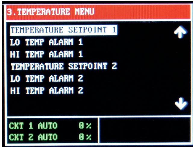
The Temperature Menu provides access to the Temperature based parameters: Temperature Setpoint, Low Temperature Alarm & High Temperature Alarm for Circuits 1 and 2 (when available).
