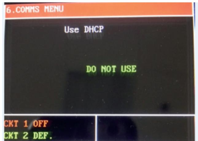
**NOTE: After pressing ENTER, power to the controller must be cycled for the change in the DHCP setting to take effect.**
