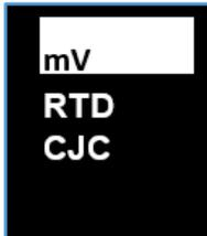
**Note:** When calibrating the RTD input type, connect an accurate 200Ω resistance source across pin 14 and pin 15, and link between pin 13 and pin 14 to replicate the 3-wire compensating lead.
