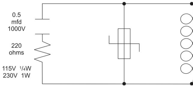
**Figure 5. Contacts:** - Arcing may occur across contacts when they open and close. This results in electrical noise as well as damage to the contacts. Connecting a properly sized RC network can eliminate this arc.
