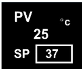
Display shows PV (process variable), units, SP (setpoint), alarm/latch statuses, error & warning messages.
