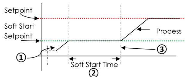
1. When powered up the unit will control to the **Soft Start Setpoint**. The control cycle time is 1/4 of the value entered (subject to the minimum possible value of 0.5s) and the maximum power demand is limited to the **Heat Power Limit** value (set in the Control menu). The reduced cycle time is used during the soft start phase.
