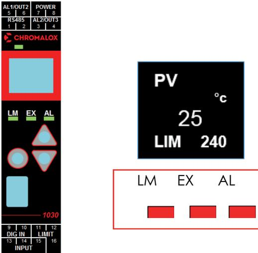
The Limiter model has fixed output functions. Depending upon which option is fitted in Output 3 it is Alarm 2 or Retransmit PV. Refer to the Information menu or check the product label identify your version.
