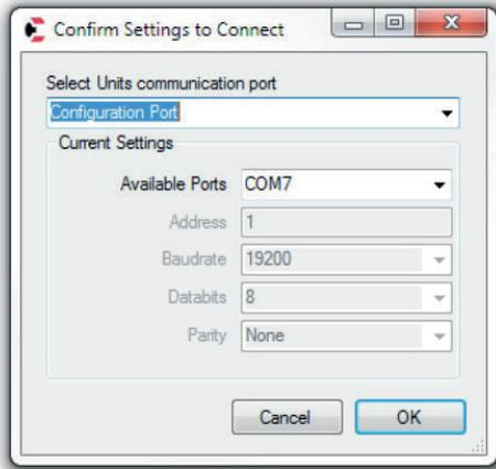
From the **Confirm Settings to Connect** window, choose which communication port (Configuration Port or RS485 Port) and the respective Port Settings (COM1 or COM7 for example). Select [ **OK** ]
