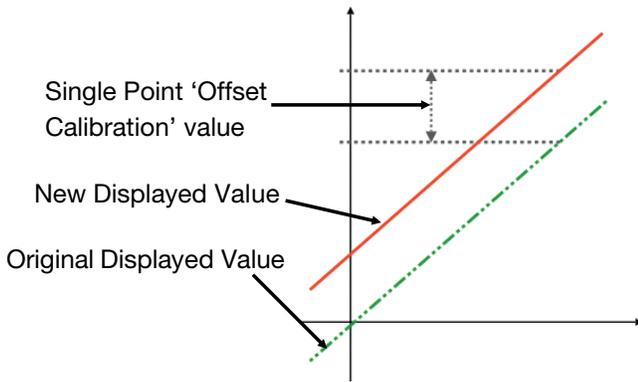
For example: If the process displays 27.8 when it should read 30, The error is -2.2 so an applied offset of +2.2 would change the displayed value to 30. The same offset is applied to all values, so at 100.0 the new displayed value would be 102.2.
