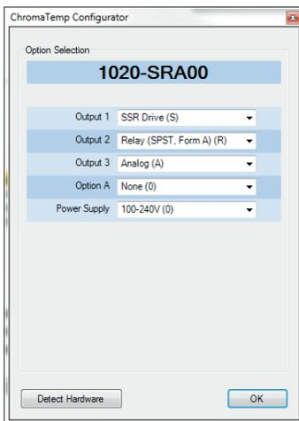
To read the settings from a DIN controller, the unit must be powered up and properly connected to your computer via the **Universal Converter**. (See 12.2 above)
