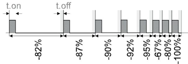
Cooling is inhibited entirely until the Minimum Cooling temperature has been exceeded. After that it turns ON with fixed duration pulses (adjustable with Impulse Length parameter). The OFF time between pulses is varied to adjust the cooling effort, but is never off for less than Minimum Off Time value whenever cooling is active. This ratio limits the maximum effective cooling.
