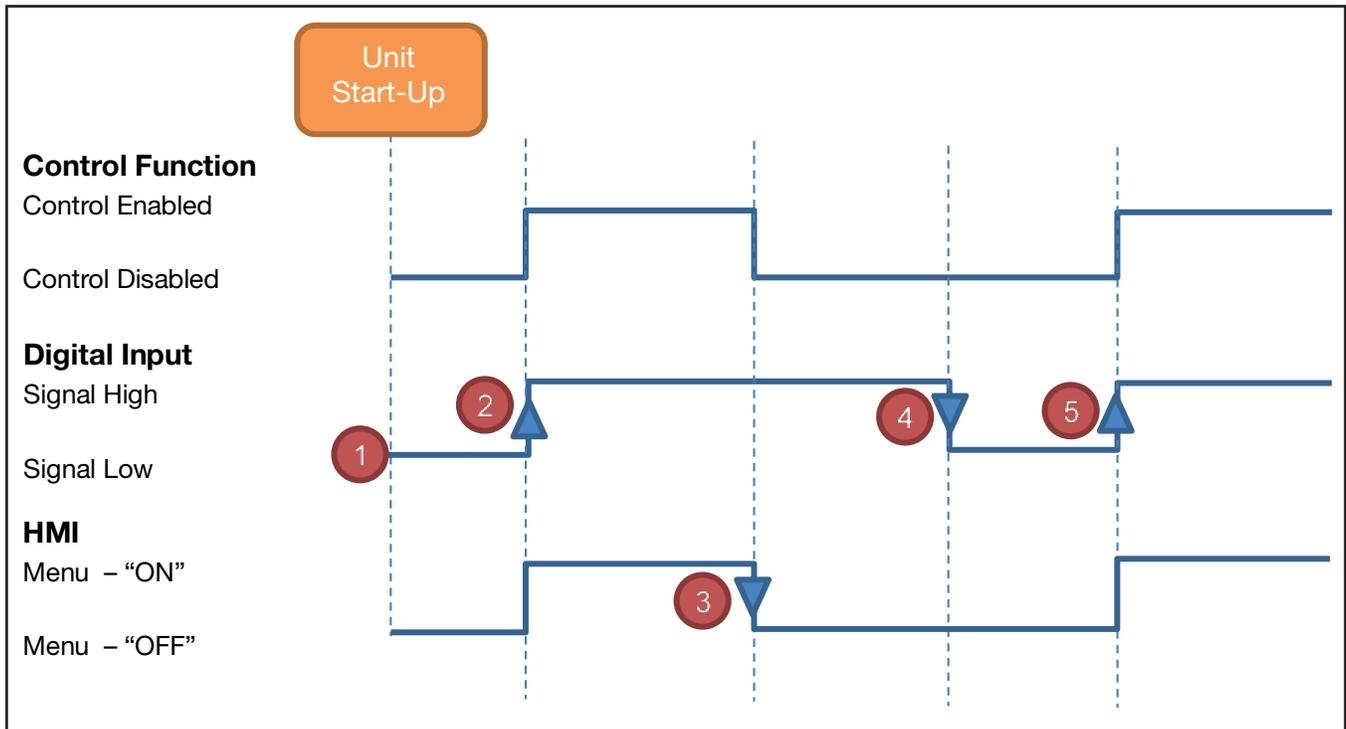
1. On start-up, the unit uses the Power-Up Action for its initial control state. In this example, it starts in the disabled condition.
