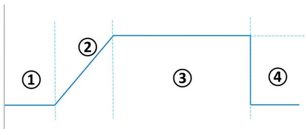
1. From power-up, if control is in the enabled state, or whenever control is changed from disabled to enabled, the unit delays process control (i.e. control is still disabled) until the Delay Timer expires (time as set by Delayed Start Time). If this is OFF, step 1 is omitted.
