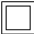
**THIS SYMBOL MEANS THE EQUIPMENT IS PROTECTED THROUGHOUT BY DOUBLE INSULATION.**
