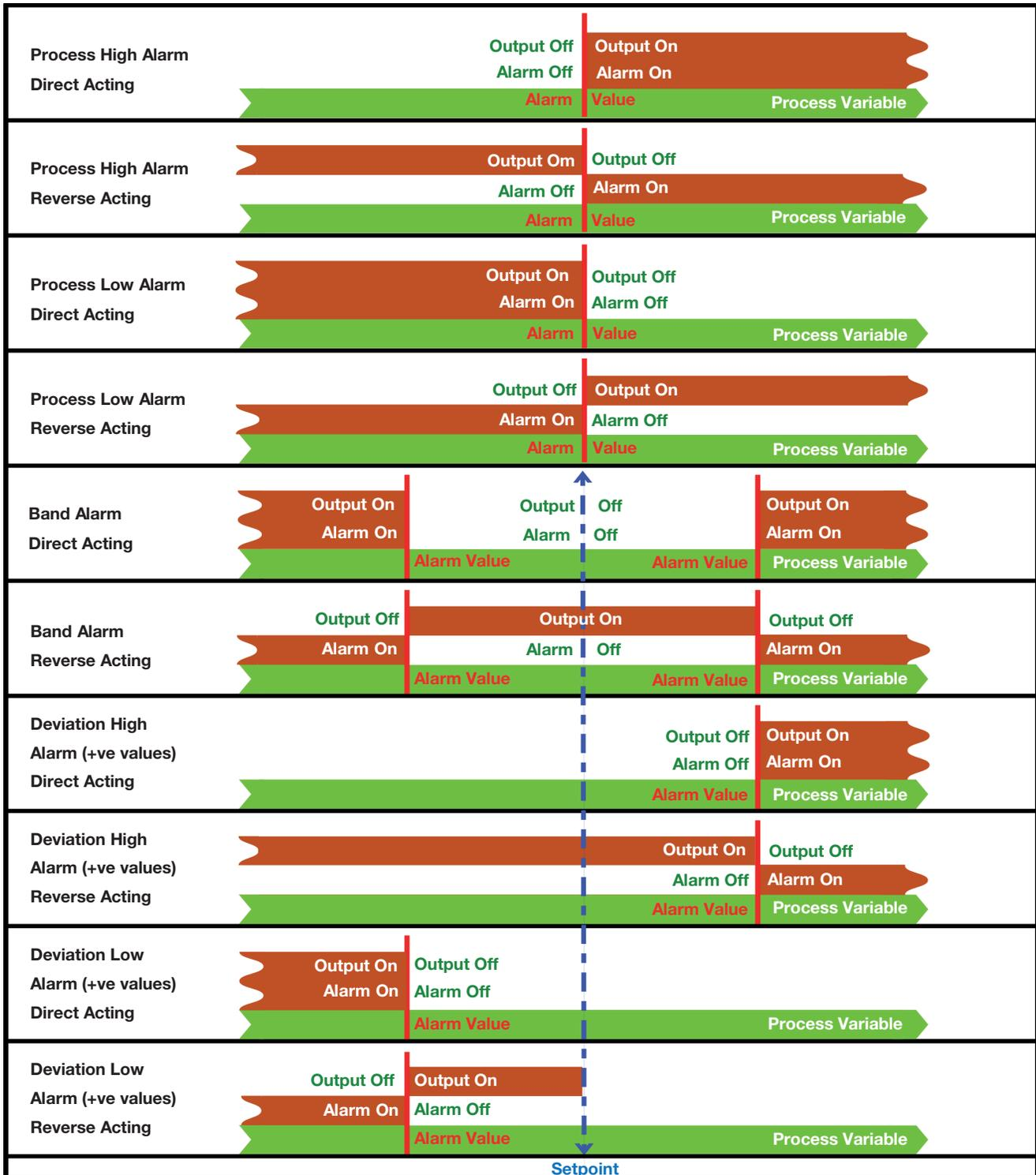
Figure 64. Alarm Operation
