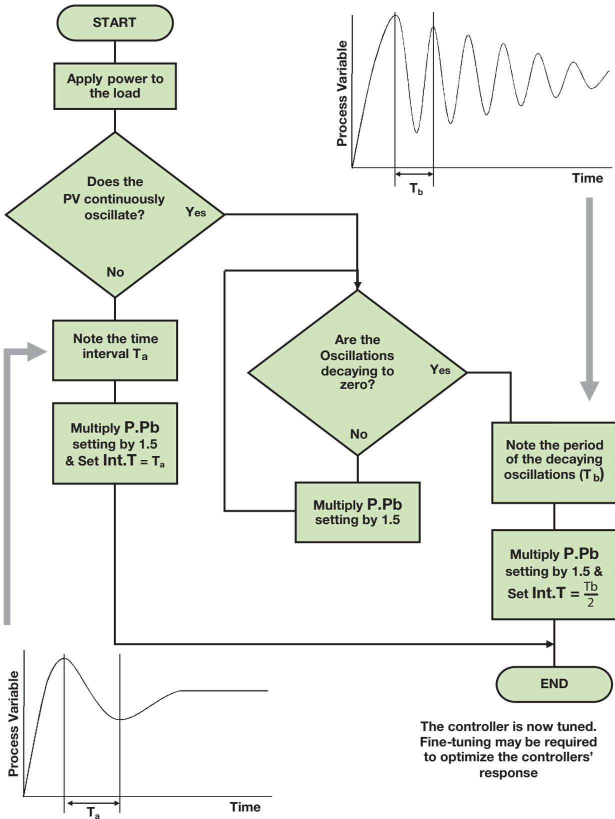
*This method can also be used to tune PID loops. Set Derivative to approx.  $T_a / 4$*
