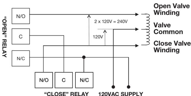
Figure 42. Interlocking of Valve Motor Drive Relays
