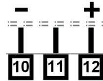
Figure 37. Plug-in Module Slot 3 - Transmitter Power Supply Module
