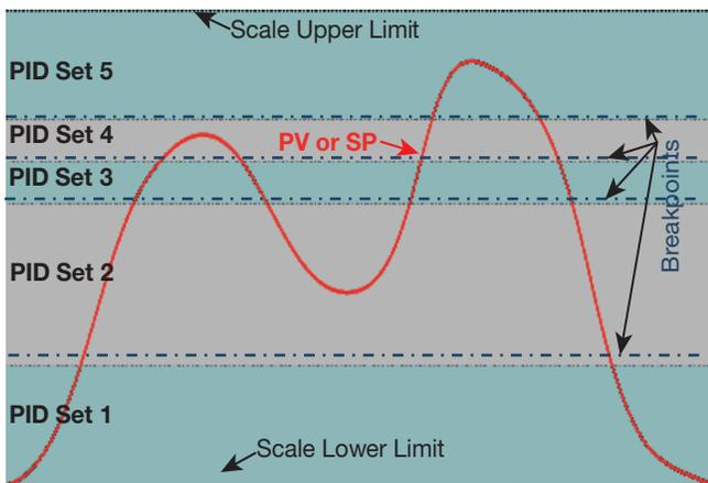
PID set 1 is used from the scaled input lower limit until the “breakpoint” for set 2 is passed and that set becomes active.
