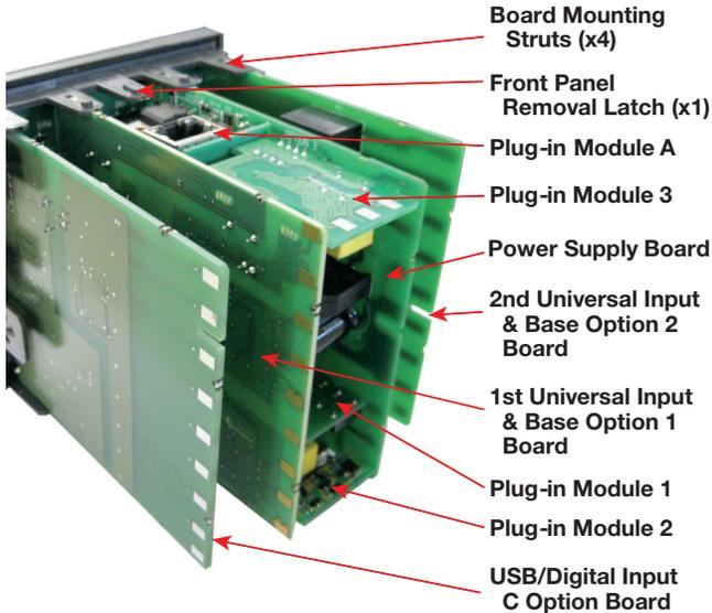
Figure 3. Rear View (uncased) & Board Positions
