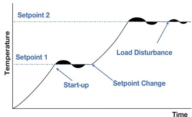
Figure 59. Self-Tune Operation
