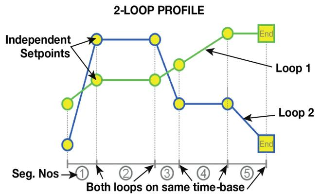
Seg. ① & ② shows a ramp and a dwell with the shared time base. The ramp direction can be different (Seg. ③), and although one loop cannot ramp while the other dwells, a “dwell” is achieved by a ramp with its final setpoint value at the same value as the previous segment (Seg. ④). Similarly, if only one loop is to Step to a new value, make the other “step” to its existing setpoint value. If you later change the previous setpoint, you may have to change both segments.
