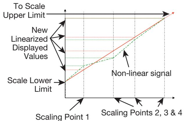
Figure 46. Multi-point Scaling
