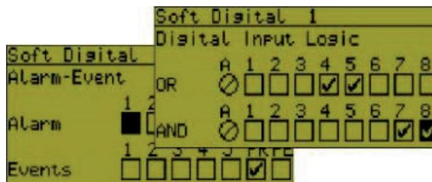
The four soft digital inputs can be configured by combining physical inputs, alarms & events using Boolean logic. Input AND selections are then globally OR'd with the input OR selections, the alarms & the events. By using the invert inputs function, NAND & NOR equivalents can be created.
