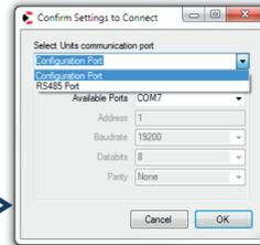
From the **Confirm Settings to Connect** window, choose which communication port (Configuration Port or RS485 Port) and the respective Port Settings. Select [ **OK** ]
