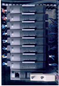
Figure 1 A typical Chromalox 1040 System The Bus Module and Loop Modules can be connected to the Bus Module, as long as the maximum of eight modules is not exceeded.
