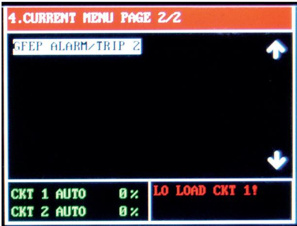
The Current Menu provides access to the current and GFEP based parameters: Low Current Alarm, High Current Alarm, GFEP Setpoint & GFEP Alarm/Trip for Circuits 1 and 2 (when available).
