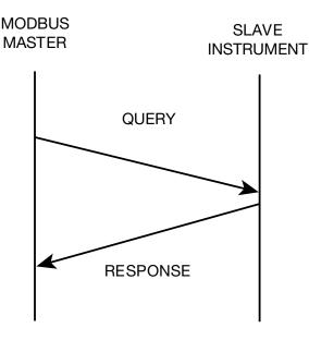
A message for either a QUERY or RESPONSE is made up of an inter-message gap followed by a sequence of data characters. The inter-message gap is at least 3.5 data character times.
