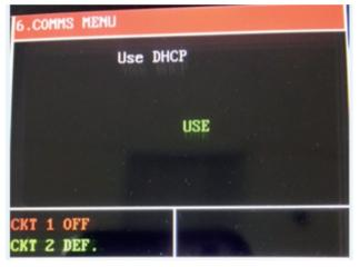
**NOTE:** After pressing ENTER, power to the controller must be cycled for the change in the DHCP setting to take effect.
