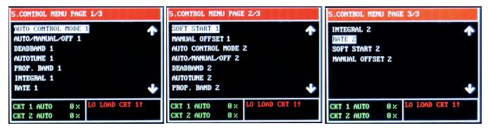
The Control Menu provides access to the types of Automatic Control, Mode of Operation, the parameters which influence the control algorithms and the Soft Start function: Auto Control Mode, Auto/Manual/Off Control, Deadband, Autotune, Proportional Band, Integral, Rate (Derivative), Soft Start function and Manual Offset.
