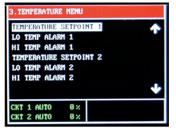
The Temperature Menu provides access to the Temperature based parameters: Temperature Setpoint, Low Temperature Alarm & High Temperature Alarm for Circuits 1 and 2 (when available).
