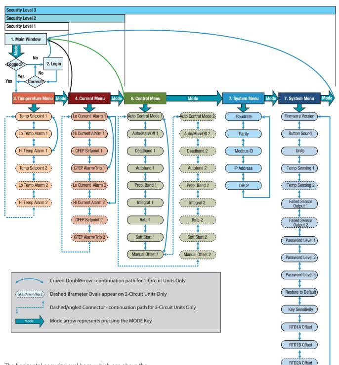
The horizontal security level bars, which are above the ITC Menu & Parameter navigation map, illustrate the available menus within that security level. The Main Window is presented when the **MODE** button is selected while the operator is at the last available menu screen within the current security level.
