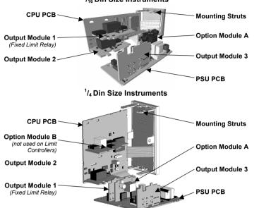
To access module A, first detach the PSU and CPU boards from the front by lifting first the upper, and then lower mounting struts. Gently separate the boards.
