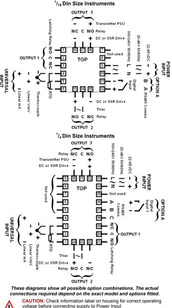
voltage before connecting supply to Power Input Fuse: 100 – 240V ac – 1amp anti-surge 24/48V ac/dc – 315mA anti-surge
