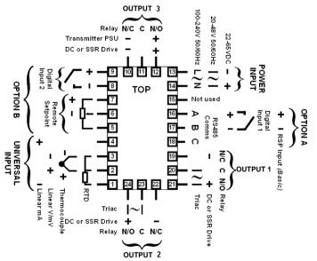
These diagrams show all possible option combinations. The actual connections required depends on the exact model and options fitted.
