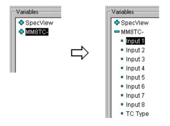
Double-click the variable you want to add to the GDW, for example, Input 1. The variable (XXX, which will be displayed as the numeric value of the variable in Runtime Mode) and its description (for example, MM8TC-, Input 1) are displayed in the top left hand corner of the GDW.
