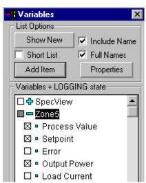
The crosses show which variables are logged. Click the box to check/uncheck each one NOTE: To include ALL the variables on a GDW in logging see the "Set All items on this GDW as Logged" menu command from the Database submenu on the Setup menu (see page 74)
