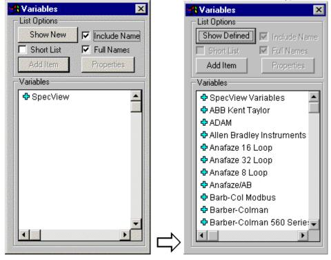
Scroll down the list of available instruments to find the name of the instrument you intend to connect. Click the symbol beside the instrument you require to display the specific instrument types. Select the appropriate one, then click **Add Item**.
