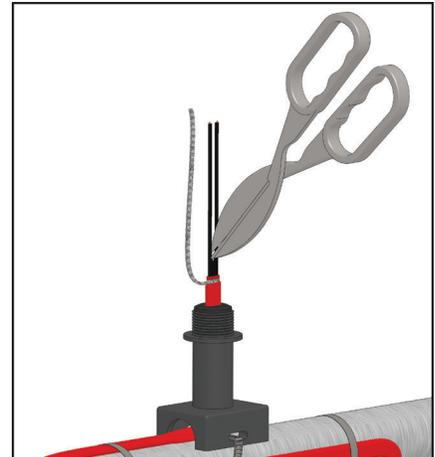
6. Use tin snips or similar tool to cut excess material from between the buss wires.
