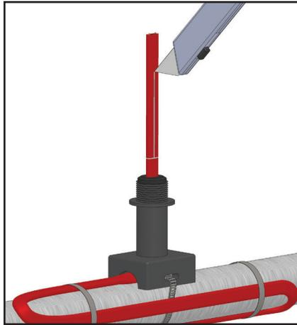
2. Score the outer insulation 7 inches from the end of the cable. Lightly cut the outer jacket up the center to the end of heating cable and remove the outer jacket from the cable. **WARNING: DO NOT CUT METAL BRAID.**
