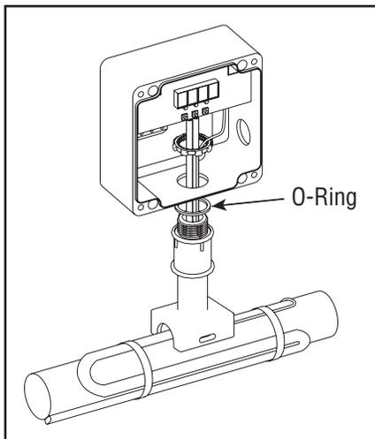
10. Seat O-Ring into compression fitting groove at base of threads. Ensure O-Ring is not twisted. Assemble junction box to compression fitting as shown. Tighten locknut until the junction box bottoms out against the lip of the compression fitting.
