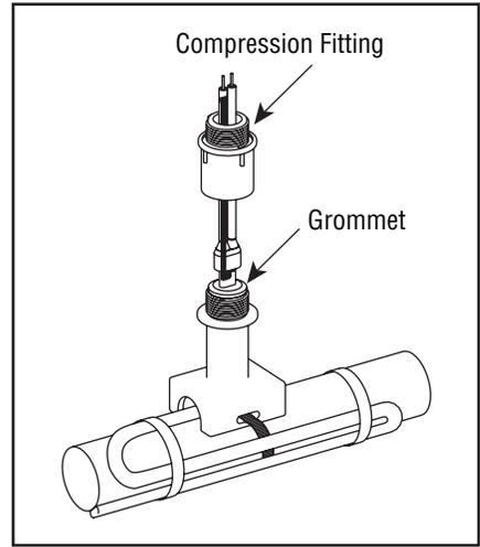
9. Slide compression fitting over cable. Grommet should be placed inside pipe standoff. Termination boot should be spaced 1/2" from sealing grommet. Tighten compression fitting until it bottoms out against pipe standoff.
