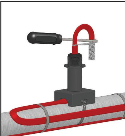
4. While bending the heating cable, work the cable through the braid opening. Pull the braid tight.
