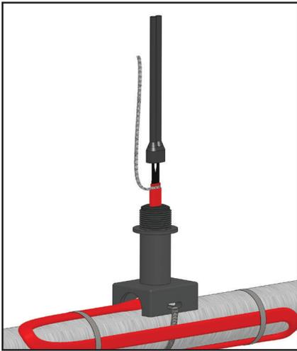
7. Liberally apply RTV over the exposed matrix and leads. Push the rubber boot over the heating cable.
