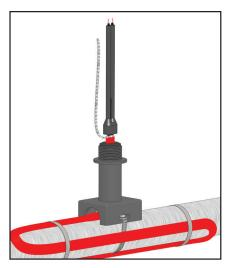
8. Strip each bus wire so that no black matrix material shows above the end of the rubber boot. Trim lead ends as needed.
