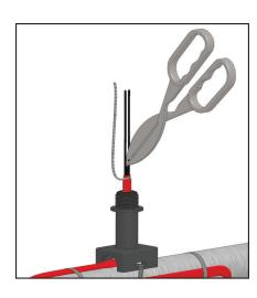
Use tin snips or similar tool to cut excess material from between the buss wires.
