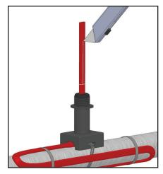
2. Score the outer insulation 7 inches from the end of the cable. Lightly cut the outer jacket up the center to the end of heating cable and remove the outer jacket from the cable. WARNING: DO NOT CUT METAL BRAID.
