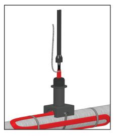
Liberally apply RTV over the exposed matrix and leads. Push the rubber boot over the heating cable.
