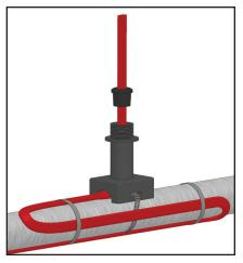
1. Insert heating cable through pipe standoff and proper grommet as shown. 8 inches of cable should extend past the grommet. Strap pipe standoff to pipe with pipe strap (Chromalox type PS not included) and attach extra cable to pipe as appropriate. If the provided RTD is to be fed through the standoff pipe, a small slice will need to be made to the outer edge of the top of the grommet. For pipes smaller than 1-1/2" diameter a small pipe adapter (Chromalox model SPA not included) is required.
