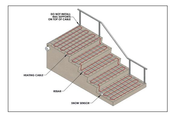
Figure 9 Typical Single Pour Detail
