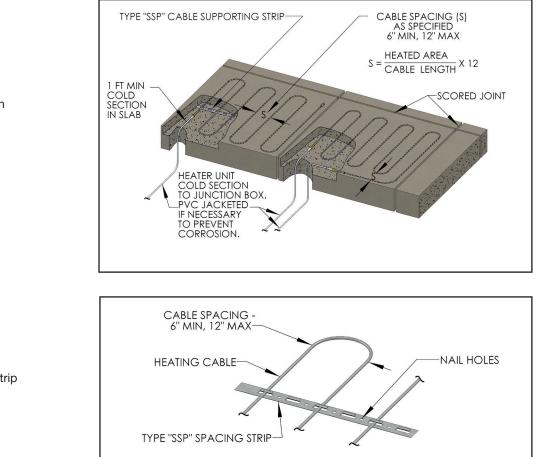
Figure 1 Typical Installation
