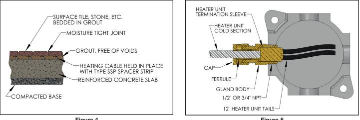
**Figure 4** Typical Detail With Cable In Grout
