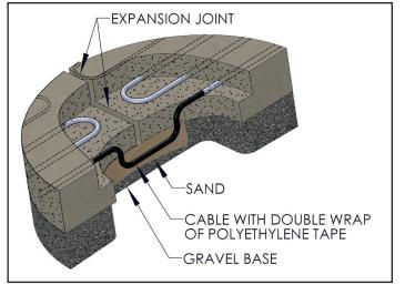
**Figure 3A** Typical Expansion Joint Detail
