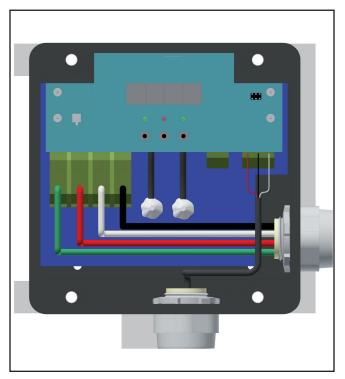
**4.** Make electrical connections to MI cable and RTD as shown. For more details on wiring connections see the DTS-HAZ installation manual (PJ944).
