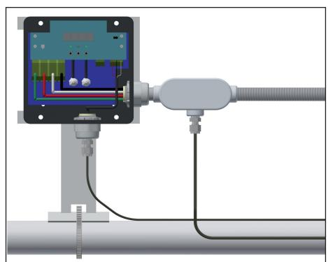
**3.** Use a CCH-2 (or equivalent) to connect tee condulet. Attach MI cable and conduit with drain.
