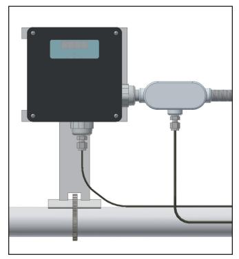
Once connections are made, place cover on box and secure the lid to the box by tightly fastening screws.
