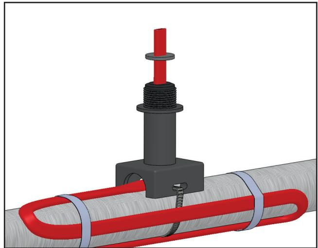
2. Place strain relief part onto cable until it is directly on top of the grommet.
