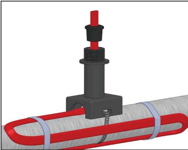
1. Insert heating cable through pipe standoff and grommet as shown. 1-1/2 Inches of cable should extend past the grommet. Strap pipe standoff to pipe with pipe strap (Chromalox type PS not included, UESL to be mounted vertically only) and attach extra cable to pipe as appropriate. For pipes smaller than 1-1/2" diameter a small pipe adapter (Chromalox model SPA not included) is required.
