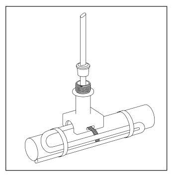
1. Insert heating cable and capillary tube through pipe standoff and grommet as shown. 8" of cable should extend past the grommet. Attach the pipe standoff to the pipe with a pipe strap (Chromalox type PS not included) as shown. Attach extra cable to pipe as appropriate. For pipes smaller than 1-1/2" diameter optional small pipe adapter (Chromalox model SPA not included) is required.
