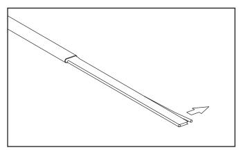
**6.** Starting at the end of the heating cable, using needle nose pliers or a knife pull each bus wire away from the core material.
