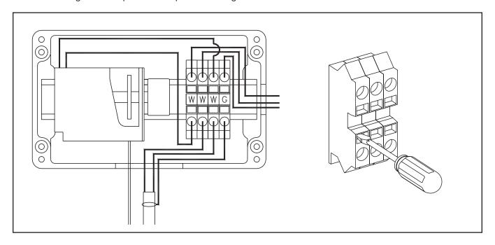
12. Attach 3/4" conduit hub. Use a flat head screwdriver to release the terminal spring clamps and insert cable leads and grounding braid. Please see the electric diagrams below for proper wiring for your application. Attach junction box cover to seal enclosure. NOTE: The conduit hub should be approved for Class 1, Div. 2; Class II Div. 1 & 2, Class III, Div. 1 & 2, and NEMA 4X rated by a nationally recognized testing laboratory.
