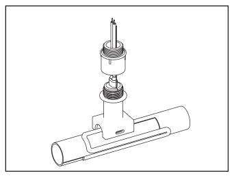
**10.** Slide compression fitting over cable. Grommet should be placed inside pipe standoff. Termination boot should be spaced 1/2" from sealing grommet.
