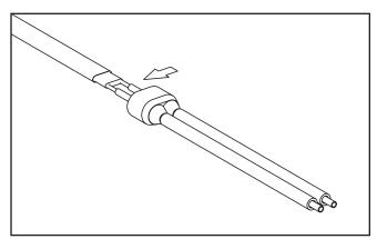
B. Liberally apply RTV over the exposed matrix and leads. Push the rubber boot over the heating cable. Trim lead ends as needed.
