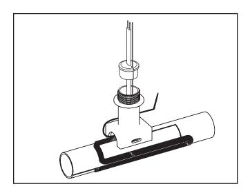
3. Insert cables and capillary tube though pipe standoff and grommet as shown. There should be 8" of
