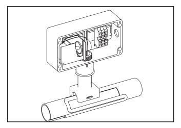
**11.** Assemble junction box to compression fitting as shown. Tighten locknut until the junction box bottoms out against the lip of the compression fitting.
