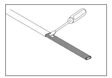
**3.** Move braid back toward the overjacket, creating a bulge. At the bulge, separate the braid to make an opening.
