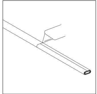
Score the outer insulation 7" from the end of the cable. Lightly cut the outer jacket up the center to the end of heating cable and remove the outer jacket from the cable. WARNING: DO NOT CUT METAL BRAID.
