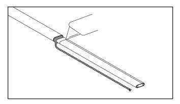
5. Score the inner insulation 6" from the end. Lightly cut the inner jacket up the center to end of heating cable and remove the inner jacket from the cable.
