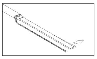
Starting at the end of the heating cable, using needle nose pliers or a knife pull each bus wire away from the core material.
