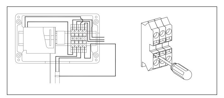
**11.** Attach conduit hub (Chromalox CCH-2 or equivalent not included). Use a flat head screwdriver to release the terminal spring clamps and insert cable leads. Supply power electrical connections should be brought to terminal as shown below. Attach junction box cover to seal enclosure.
