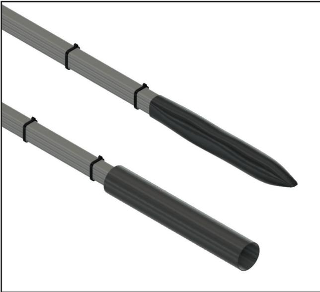
15. Place the heat shrink tube over the connection, allowing about 1-1/2" of empty space in the end of the tube. Use a heat gun to completely shrink the tube. Pinch the end of the shrunk tube with needle nose pliers and ensure the end is fully sealed.
