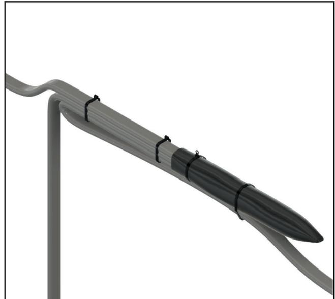
16. Attach the clamp tie to the center of the connection. Fold the bottom heating cable under and secure to the connection with a third cable tie. Attach the connection to the top of the gutter and away from the flow path of the melt water using the clamp tie.
