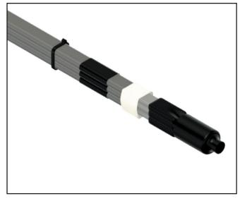
**13.** Place the insulated barrel connectors over each set of bus wires. Use a crimping tool to crimp each set together.
