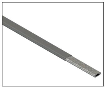
Score the cable outer jacket 2" from the cable end, being careful not to damage the braid or the base cable insulation. Remove the jacket to expose the braid.
