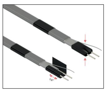
**6.** Remove release paper from mastic and place mastic tape around the end of the cable. Position as shown. Pinch in the center of the bus wires to completely seal.
