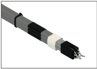
**12.** Twist each set of bus wires together. **Do not twist bus wires from the same cable together.**
