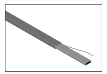
3. Pick the braid apart near the outer jacket and pull the cable through the opening in the braid. Twist the braid into a pigtail on the same side of each cable.
