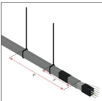
8. Once the cables are aligned, fasten them with cable ties at the positions shown.
