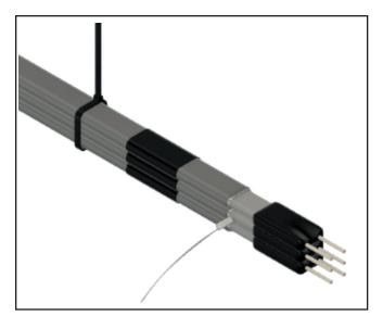
**9.** Twist all three braid pigtails together. Slide the uninsulated crimp over the braid as shown.
