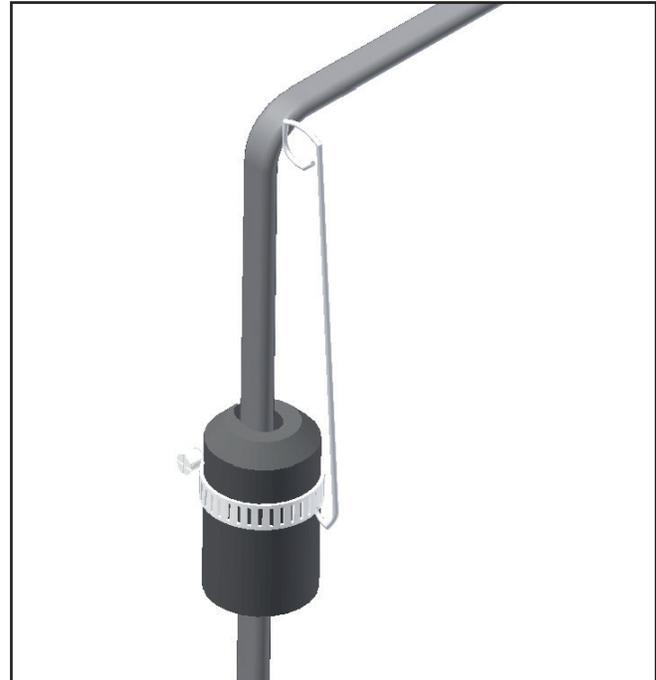
**2.** The wire hanger has a 180° hairpin bend at one end and a loop bend at the other end. Center the hairpin end of the wire hanger along the grommet. Slide the clamp over the wire hanger and into the bend of the hanger. Tighten the clamp until the hanger and cable are firmly
