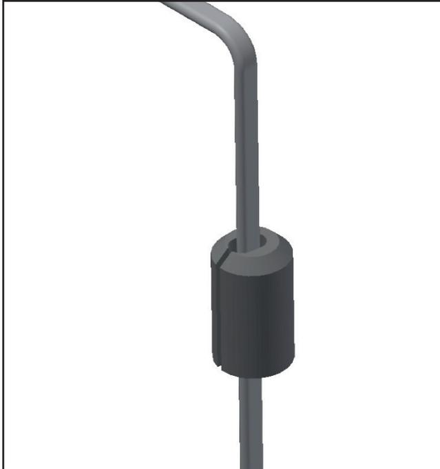
**1.** Place the split grommet around the heating cable where the downspout hanger will be placed.
