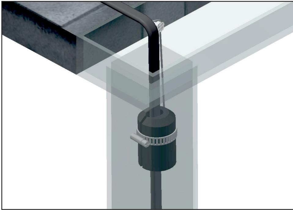
3. Attach the hanger assembly to the roof by driving a roofing nail or screw through the looped end of the hanger.
